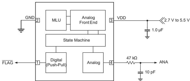
Figure 6: Complete Schematics for CT220
