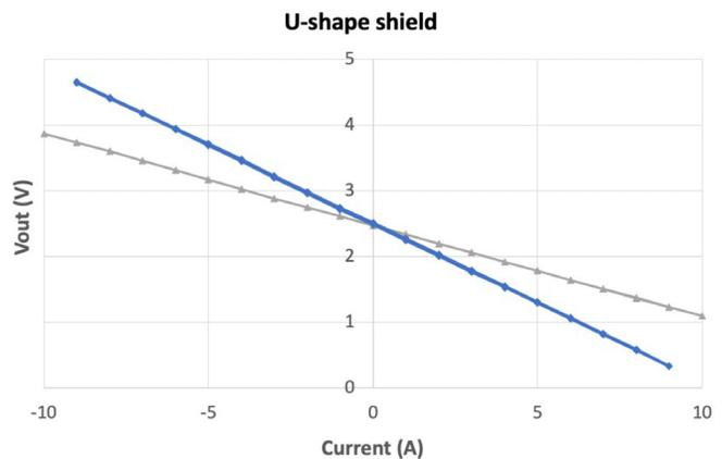
Figure 20: U-Shield Performance Against External Magnetic Fields.
