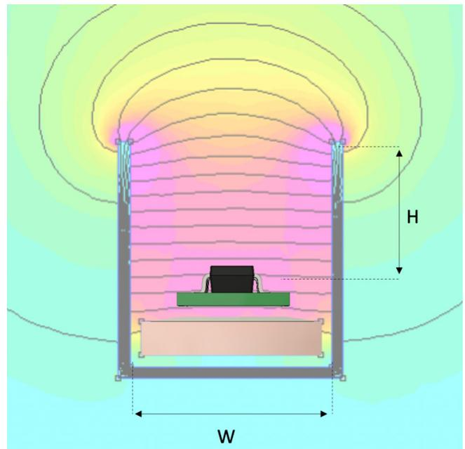
Figure 5: Magnetic Field Lines With a Shield
