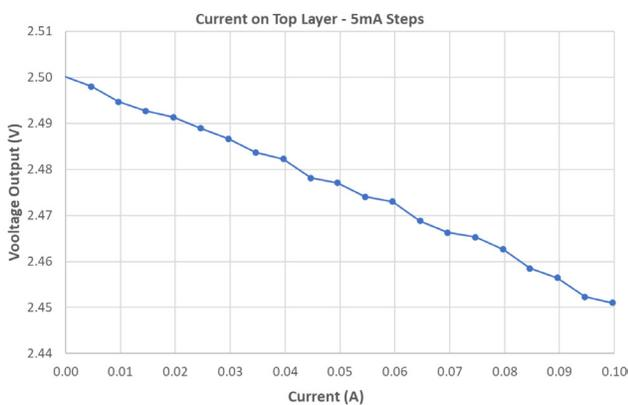
Figure 12: Resolution Achieved Using Top Copper Layer
