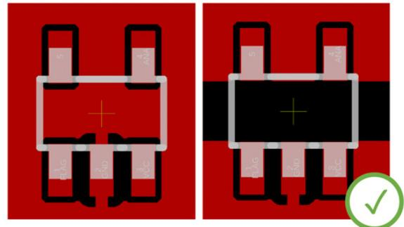
Figure 8: Recommended PCB Layout for CT220
