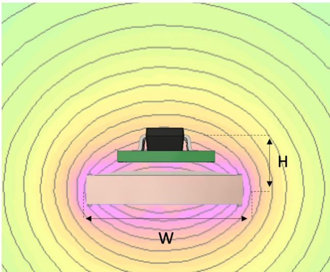
Figure 4: Magnetic Field Lines Without a Shield
