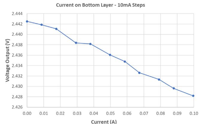
Figure 14: Resolution Achieved Using Bottom Copper Layer
