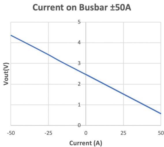
Figure 16: Resolution Achieved Using Busbar
