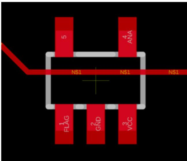
Figure 7: Poor PCB Layout for CT220
