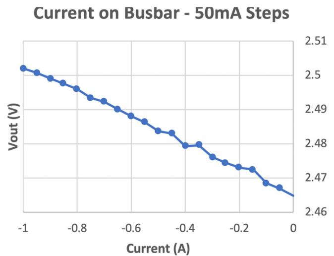
Figure 17: Resolution Achieved Using Busbar
