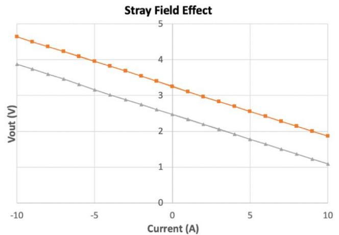
Figure 18: Offset Generated by External Stray Field
