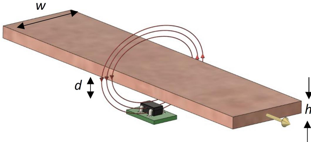
Figure 15: Current Flowing on the Busbar ( $d = 4.0$  mm,  $w = 12.7$  mm, and  $h = 1.59$  mm)
