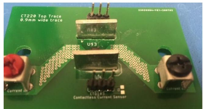
Figure 19: U-Shield on CTD221 Evaluation Board
