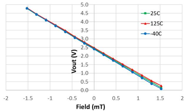
Figure 1: Voltage Output vs. Magnetic Field Under Different Temperature Levels
