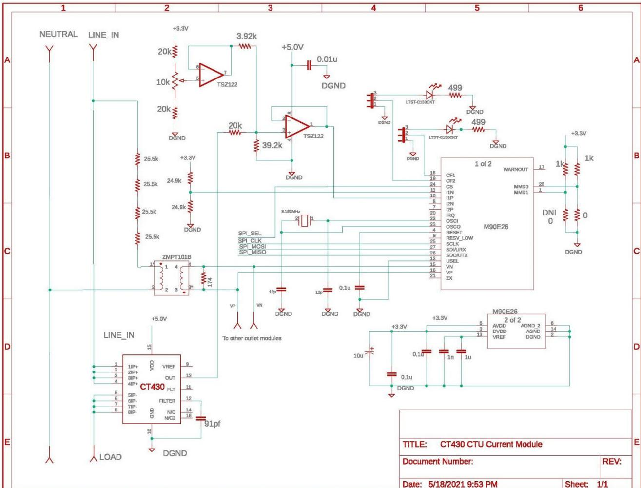
Figure 6: CT430 PDU Outlet Module
