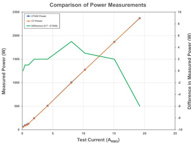
Figure 3: Power Measurement Comparison
