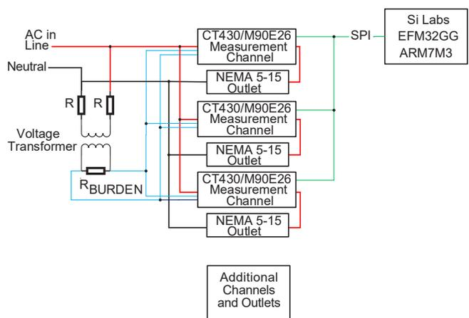
Figure 2: PDU Evaluation Board Block Diagram
