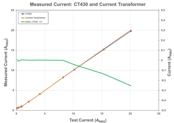
Figure 4: Current Measurement Comparison
