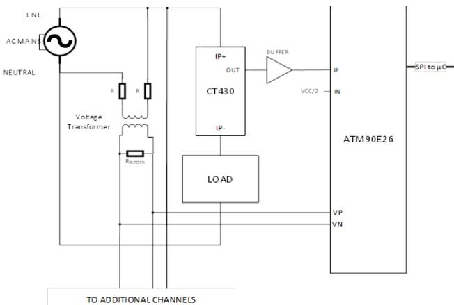
Figure 1: PDU Channel Architecture
