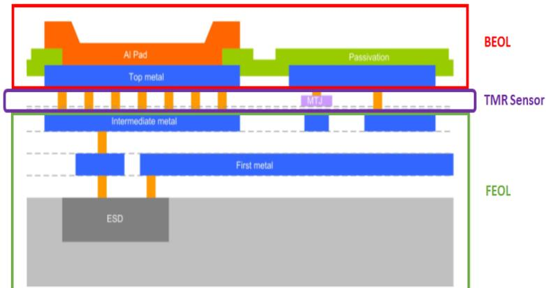
Figure 9: XtremeSense TMR construction
