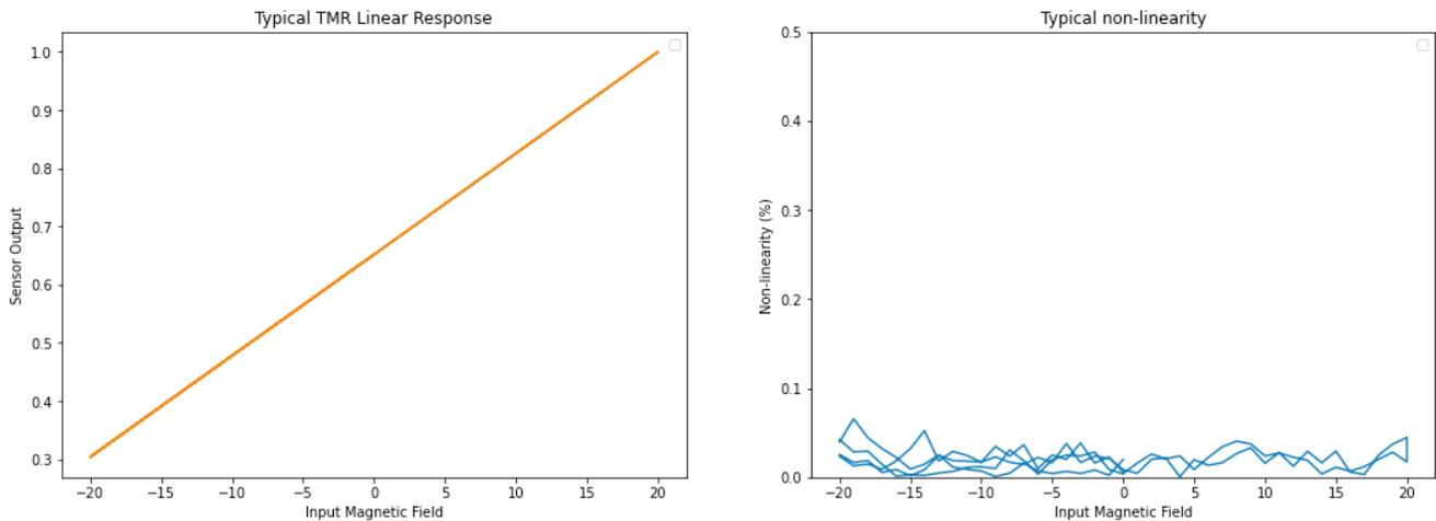
Figure 3: XtremeSense TMR linearity error
