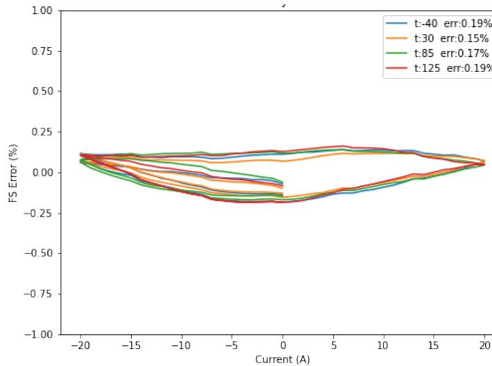
Figure 5: Ferromagnetic concentrators generate magnetic hysteresis
