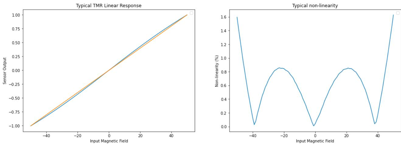
Figure 2: Typical TMR linearity error
