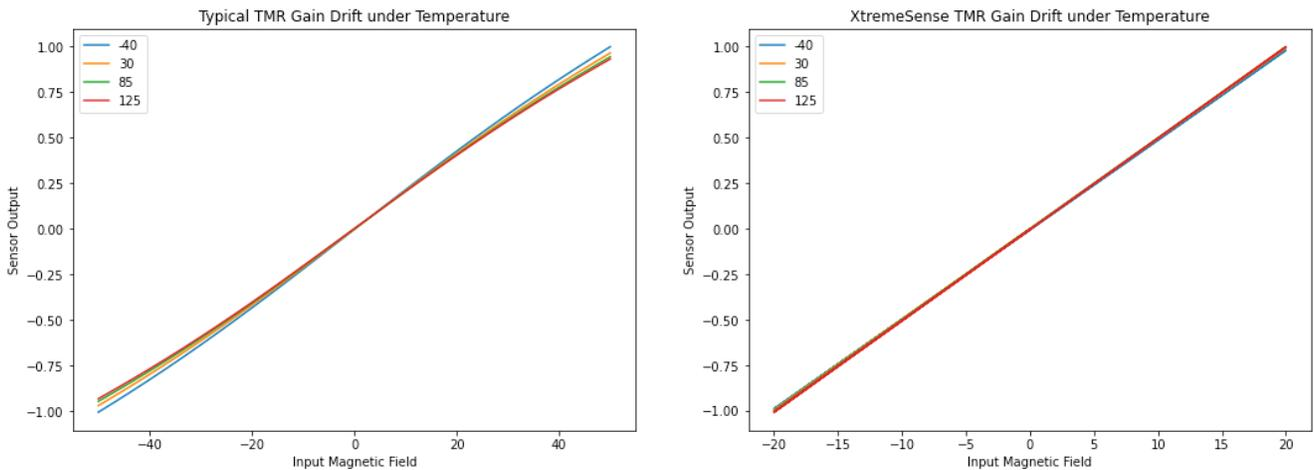
Figure 8: Gain drift under temperature
