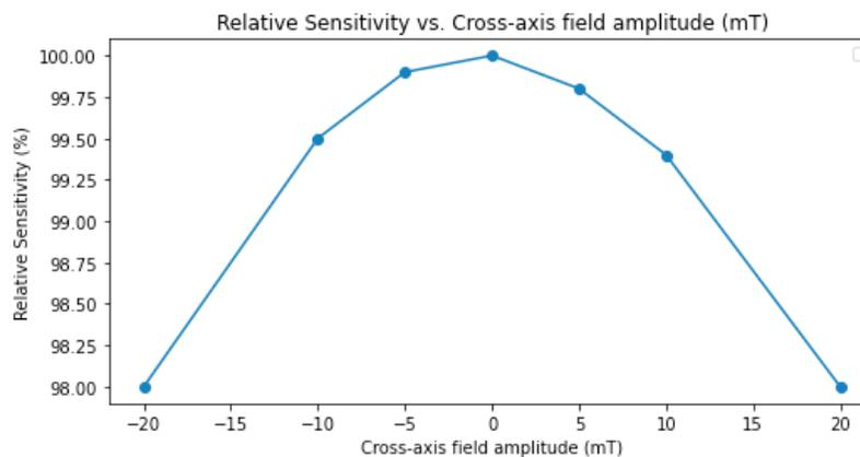
Figure 6: Relative sensitivity vs Cross-axis field amplitude
