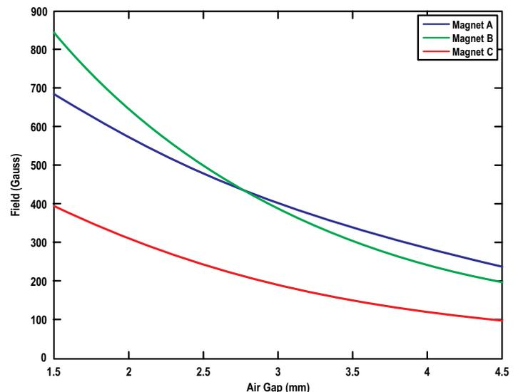
Figure 8: Magnet Field Regarding the Air Gap of the Three Magnets
