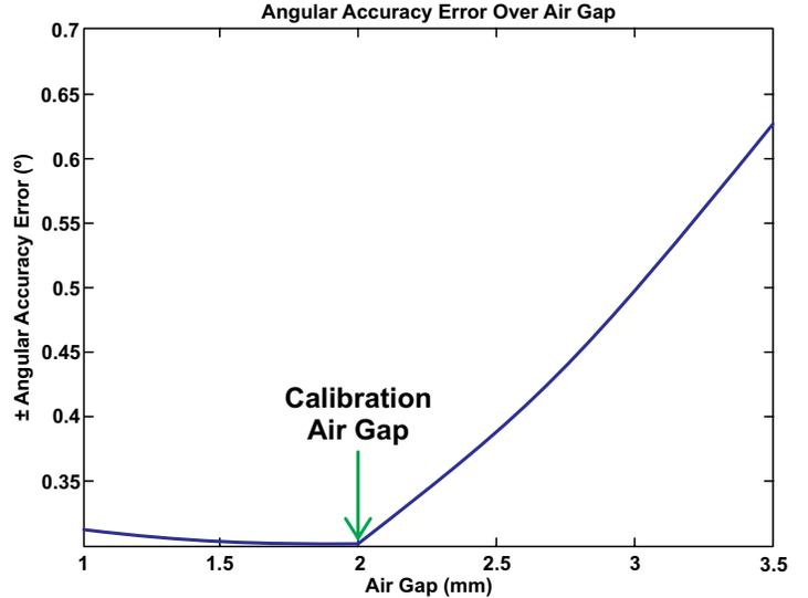
Figure 11: Magnet C, Angular Accuracy Error vs. Air Gap
