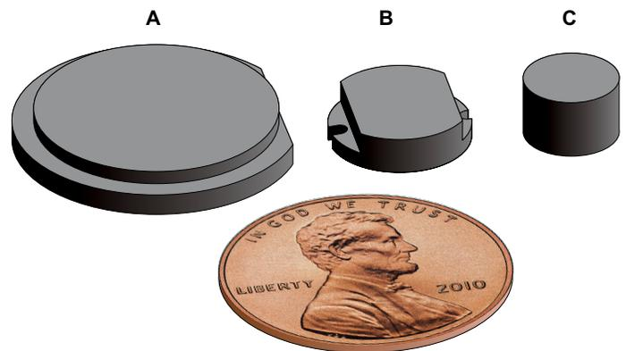
**Figure 5: Size Comparison of the Three Magnets Selected**
