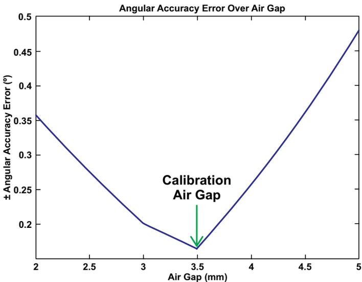
Figure 10: Magnet B, Angular Accuracy Error vs. Air Gap
