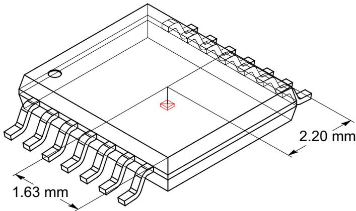
**Figure 3: CVH Transducer Placement in the TSSOP 14 Package**
