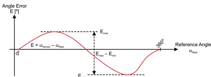
Figure 7: Angle Error and Accuracy Error Definition
