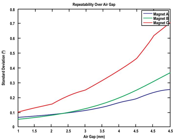
Figure 17: Standard Deviation of Angle Readings on Magnets A, B, and C vs. Air Gap<sup>4</sup>
