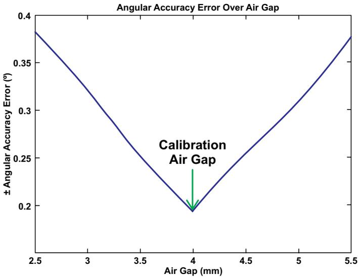
Figure 9: Magnet A, Angular Accuracy Error vs. Air Gap
