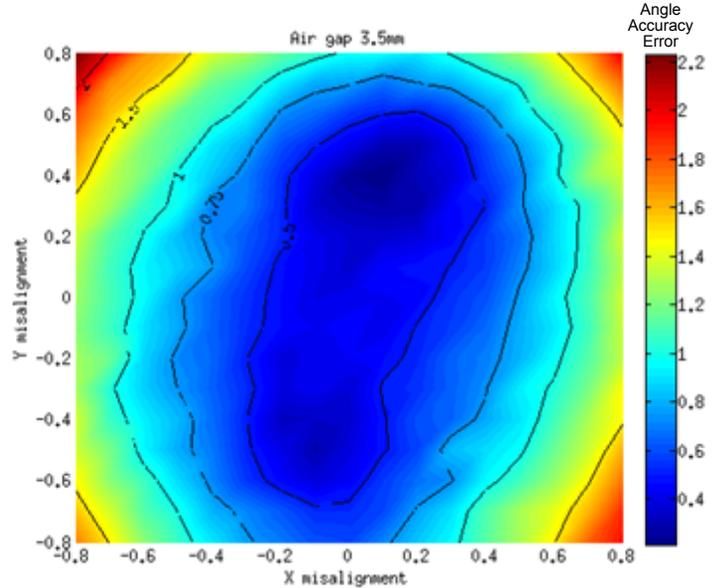
Figure 13: Angular Accuracy Error of Magnet B at 3.5 mm Air Gap
