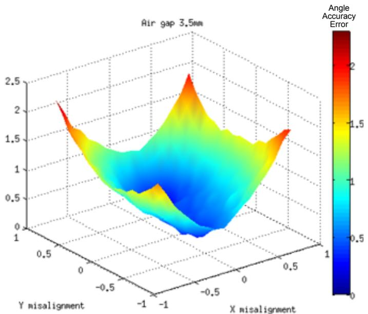
**Figure 15: Angular Accuracy Error of Magnet B at 3.5 mm Air Gap**
