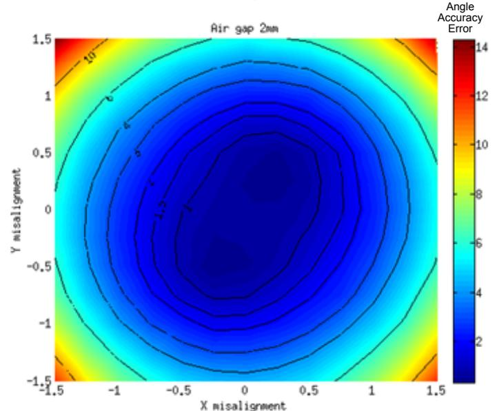
Figure 14: Angular Accuracy Error of Magnet C at 2 mm Air Gap
