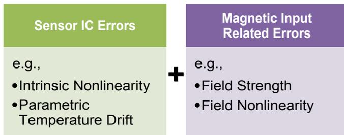
**Figure 1: Angle Measurement Errors and Their Origins**
