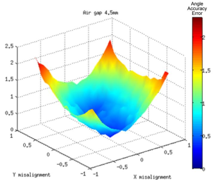
**Figure 16: Angular Accuracy Error of Magnet B at 4.5 mm Air Gap**
