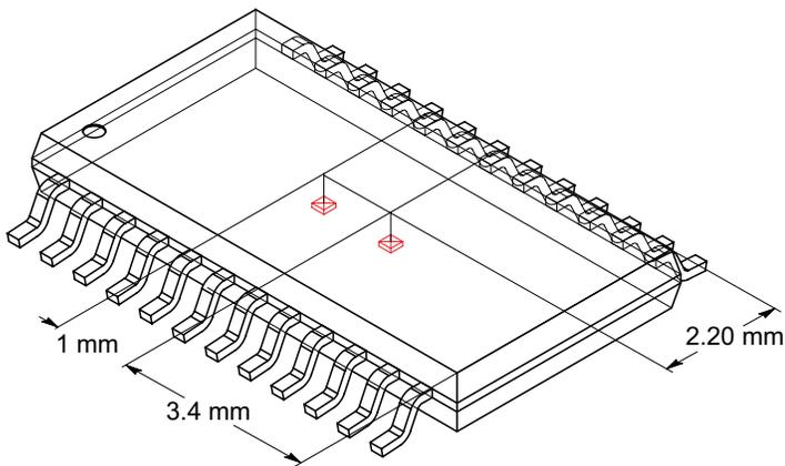
**Figure 4: CVH Transducer Placement in the TSSOP 24 Dual Die Package**
