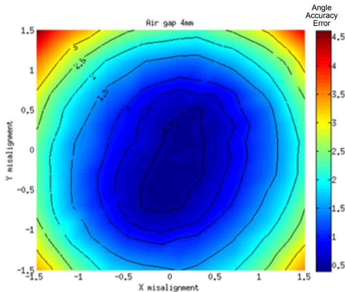
Figure 12: Angular Accuracy Error of Magnet A at 4 mm Air Gap
