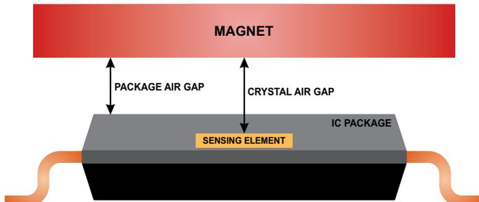
Figure 6: Air Gap Definition
