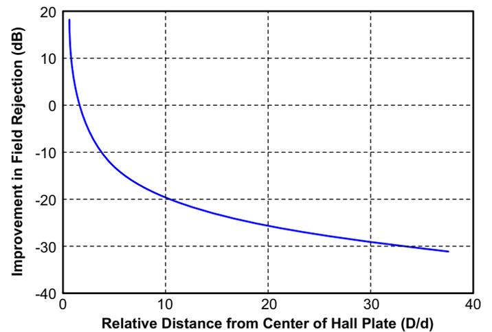
**Figure 8: Rejection Ratio of Single Hall vs. Differential Hall Configuration Over the Relative Distance of the External Wire from the Sensor IC (D/d)**
