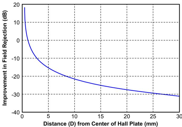
**Figure 7: Rejection Ratio of Single Hall vs. Differential Hall Configuration Over the Distance of the External Wire from the Sensor IC**
