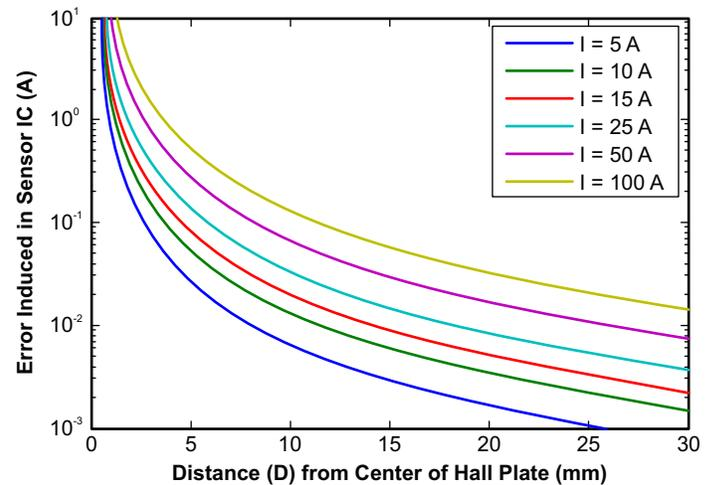
**Figure 6: Error (A) vs. Distance from Current Carrying Wire for Differential Sensing with Current Flowing Perpendicular to Hall Plates (d is 0.8 mm)**
