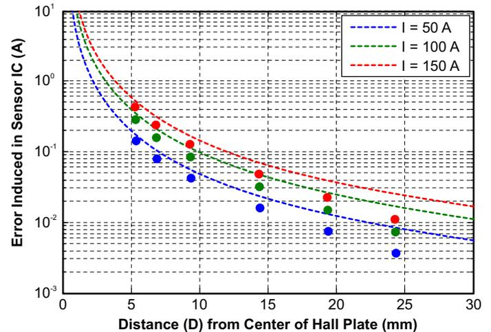
Figure 10: Estimated Error (A) vs. Distance from Current Carrying Wire for Differential Sensing
