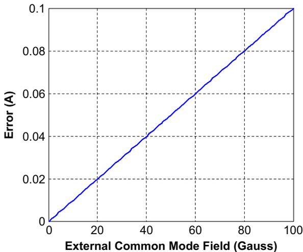
**Figure 3: Error (in Amperes) vs. Common Mode Field Due to 1% Mismatch in the Two Hall Plates.**
