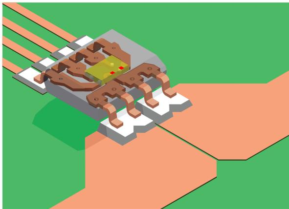
Figure 1: ACS724 Integrated Current Sensor IC [4]
