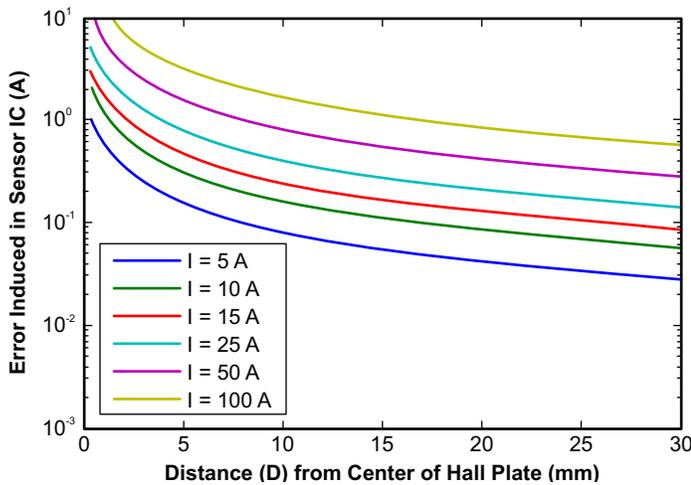
**Figure 5: Error (A) vs. Distance from Current Carrying Wire for Single Hall Sensing (d is 0.8 mm)**
