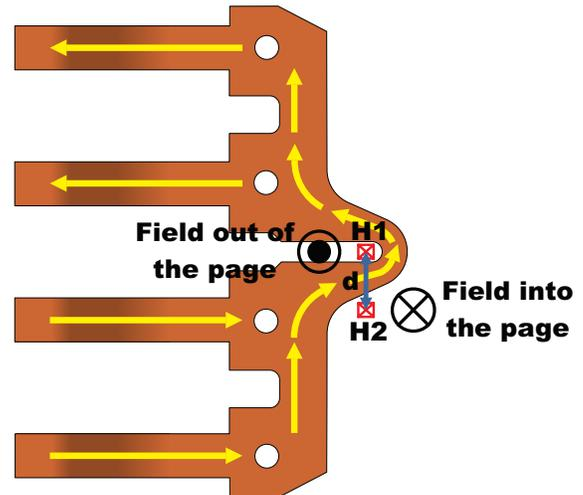
Figure 2: Integrated Current Sensor IC Leadframe with Differential Hall Plate Configuration
