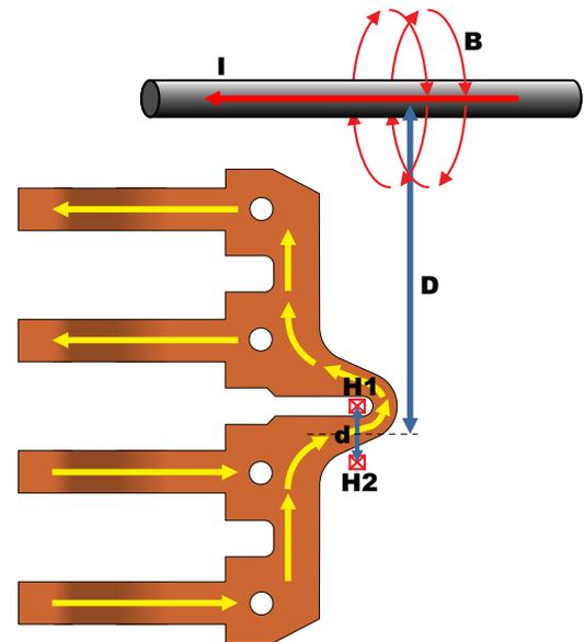
**Figure 4: External Current Flow Perpendicular to the Two Hall Plates**
