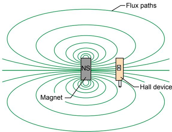
Figure 53. Typical magnetic field generated as magnetic flux passes through free air, with only a small portion passing through the Hall device
