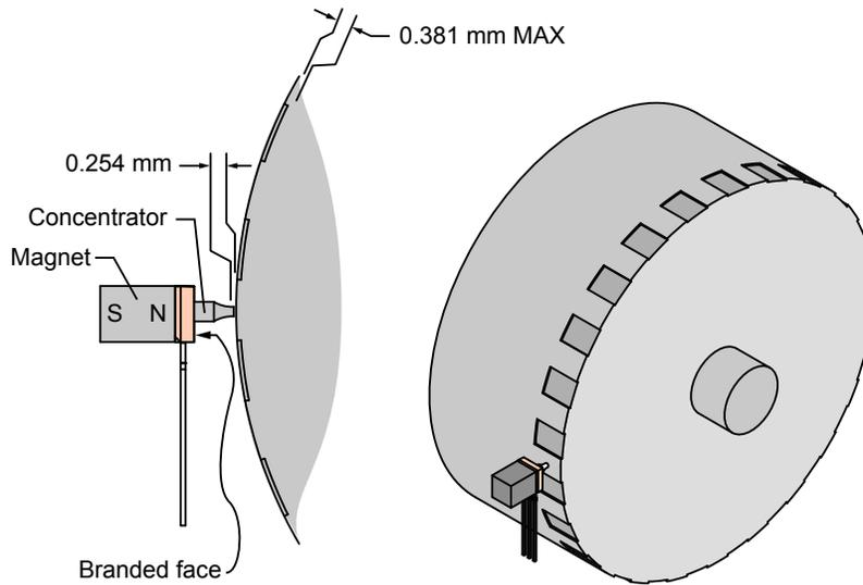
Figure 71. Demonstration of printer drum monitoring application
