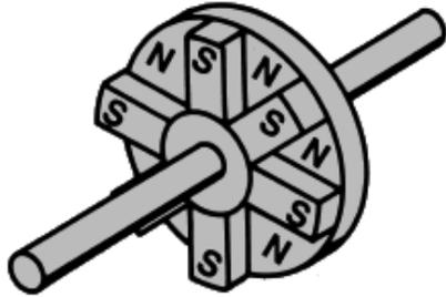
Figure 29. Demonstration of assembled inexpensive ring magnet
