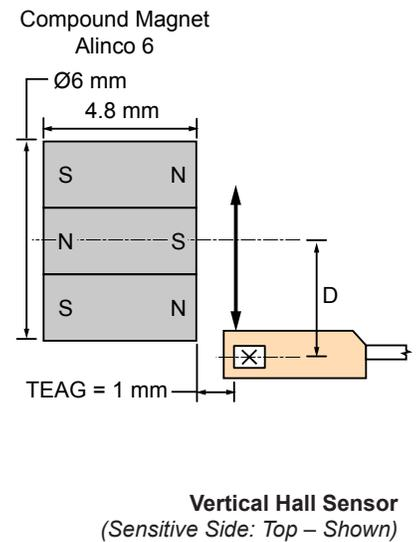
Figure 52. Example of slide-by motion, magnets on one side, compound magnets
