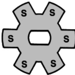
Figure 27. Demonstration of rubber magnet stock layout for inexpensive ring magnet
