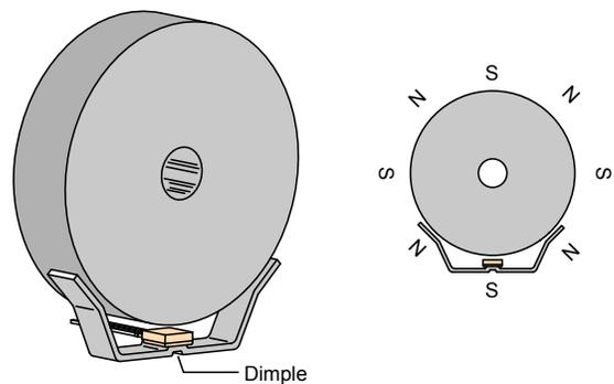
Figure 59. Demonstration of mesa-type bracket and flux concentrator
