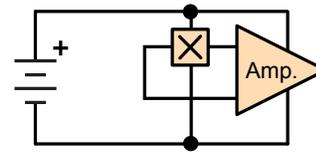
Figure 4. Hall circuit with amplification of  $V_{HALL}$
