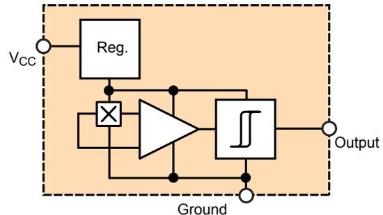
Figure 6. Hall circuit with digital output capability
