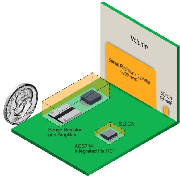
Figure 2. PCB volume comparison of typical Hall current sensor ICs versus traditional sense resistance and operational amplifier current sensing
