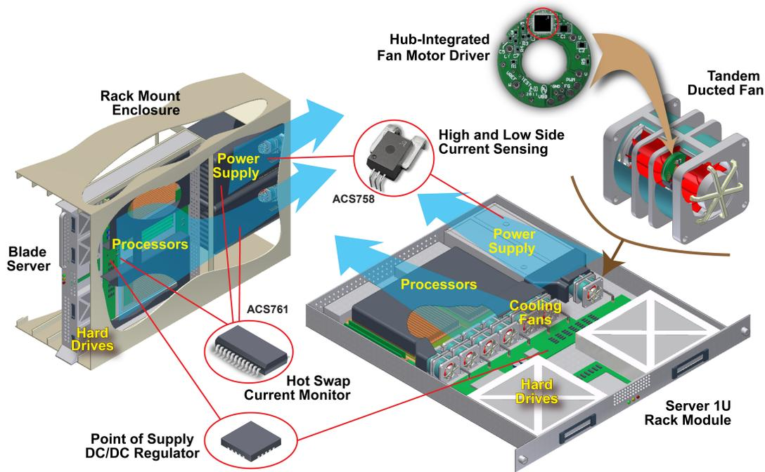
Figure 1. Fan-management, current-sensing, hot-swap-management, and PoS-regulation applications in standard rack-mount and blade servers.
