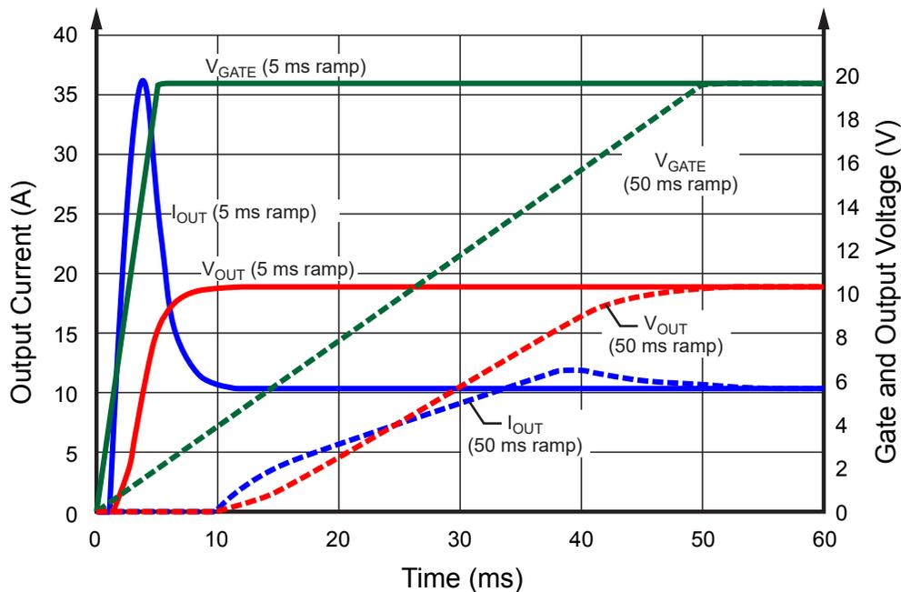
Figure 3. Hot-swapping current-surge suppression simulation
