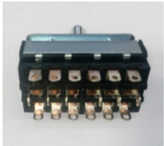
Figure 3: A six-pole, double-throw switch showing front view (left) and rear view (right)
