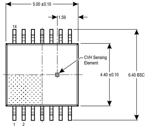
Figure 7: CVH Location within the A1335 Single-Die IC
