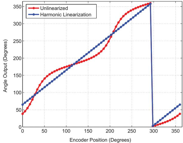
**Figure 13: Sensor output pre- and post-linearization. Note that this plot is before “Zero Position” programming, and 295 degrees from the encoder corresponds to zero degrees of Angle Output (A1335 IC output signal).**
