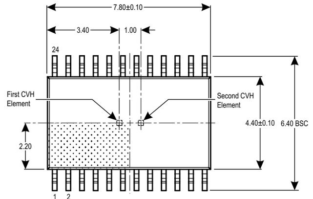
Figure 8: CVH Location within the A1335 Dual-Die IC
