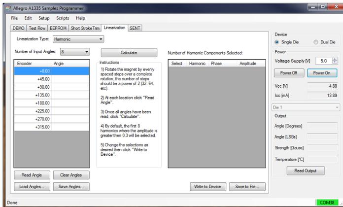
Figure 9: Linearization Tab
