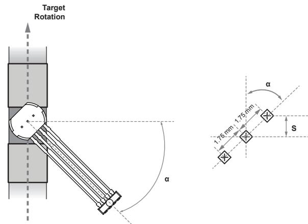
Figure 9: Sensor Twist in Front of the Target
