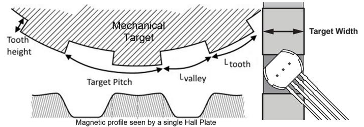
Figure 3: Target Parameters
