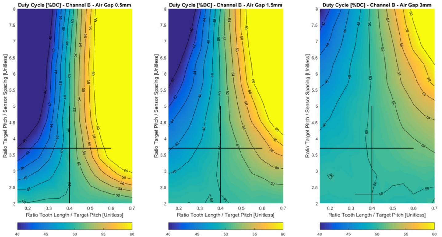
Figure 8: Duty Cycle on Channel B at 0.5 mm, 1.5 mm, and 3.0 mm Air Gap
