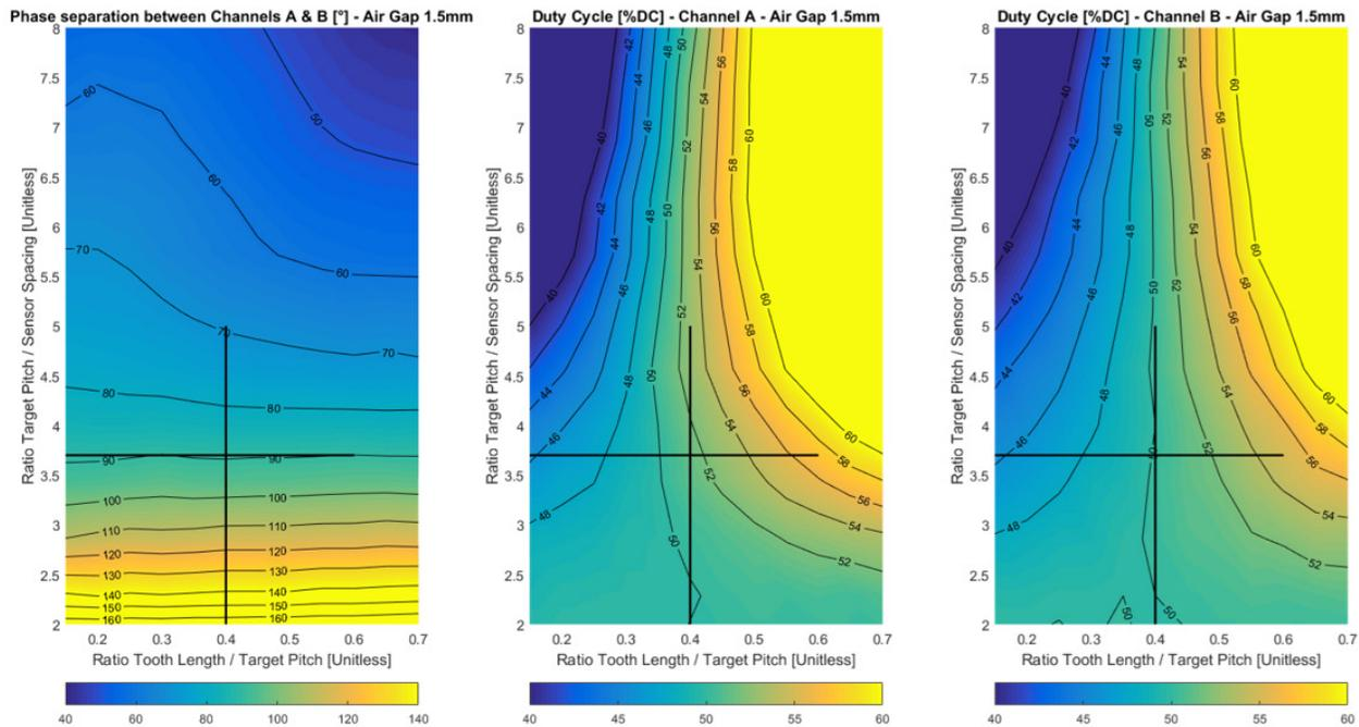
Figure 5: Phase Shift and Duty Cycle at 1.5 mm
