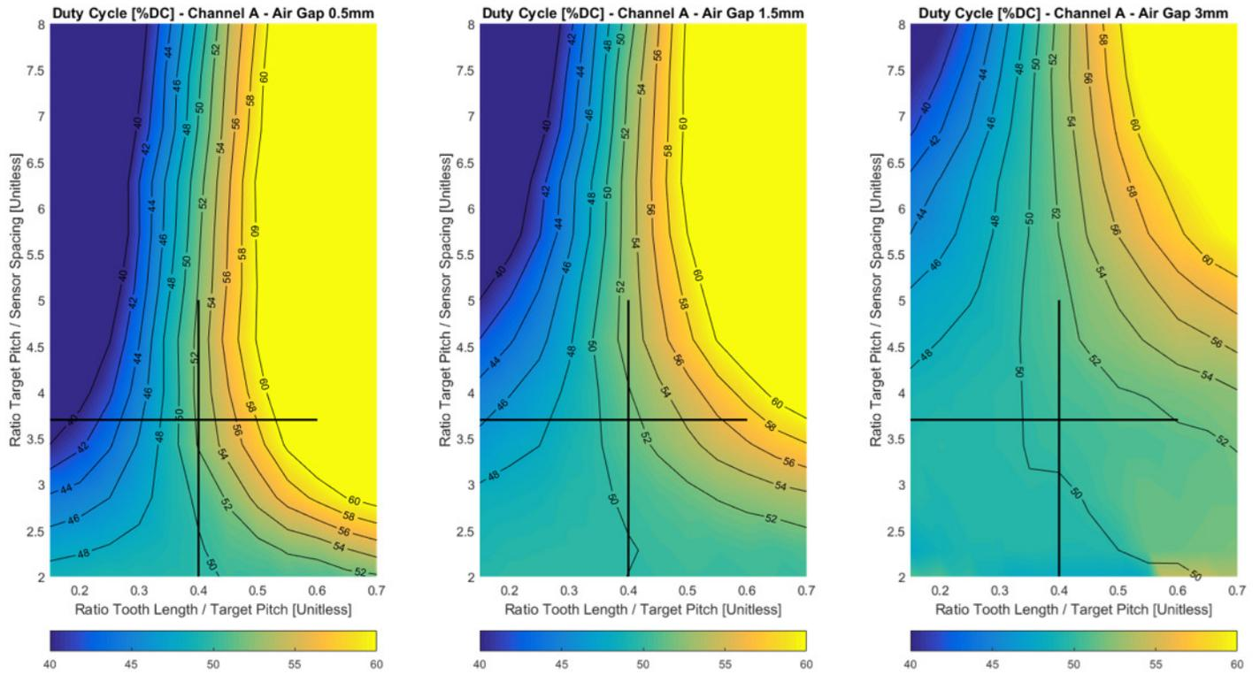
Figure 7: Duty Cycle on Channel A at 0.5 mm, 1.5 mm, and 3.0 mm Air Gap
