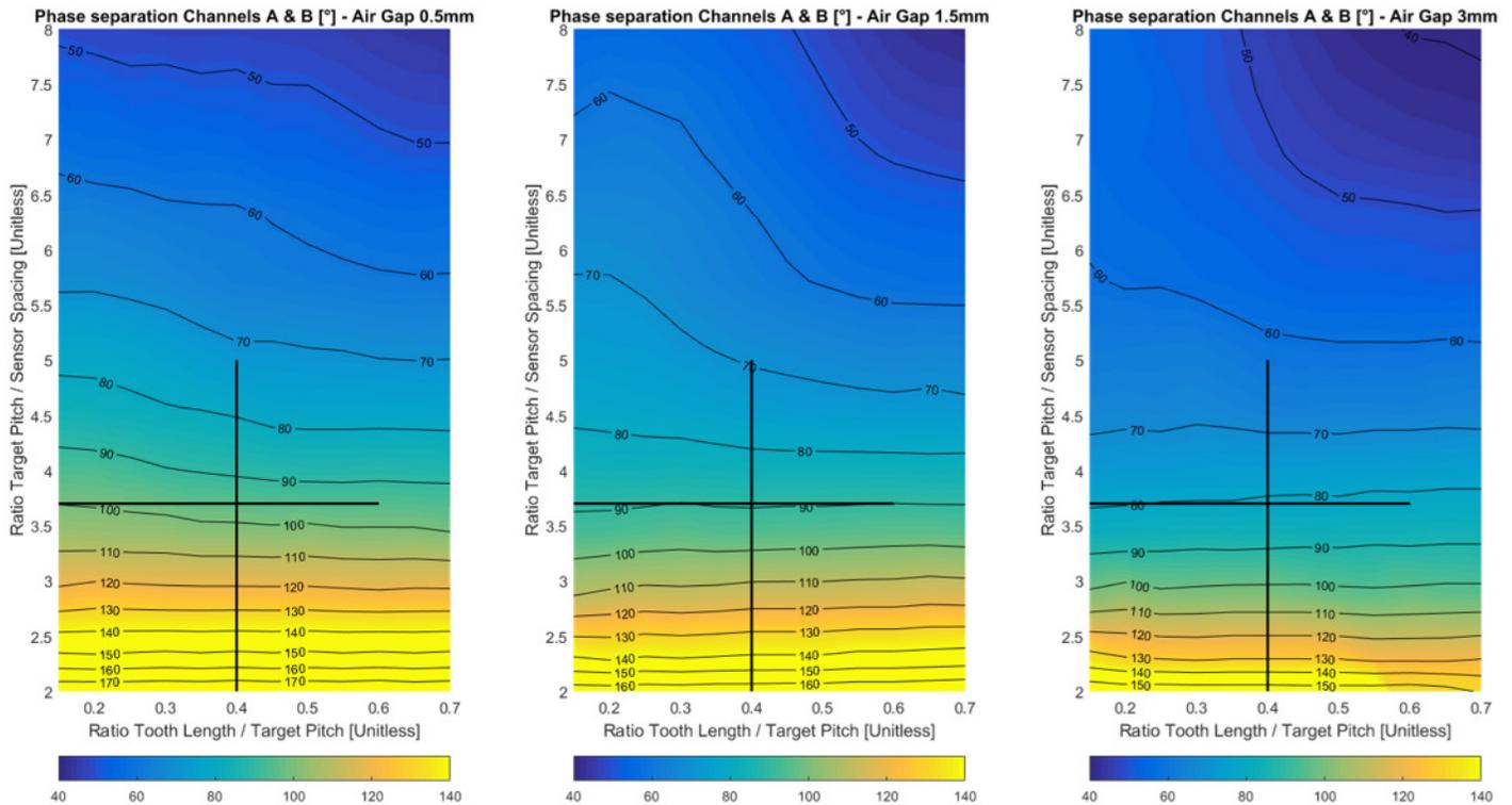
Figure 6: Phase between Channel A and B at 0.5 mm, 1.5 mm, and 3.0 mm Air Gap
