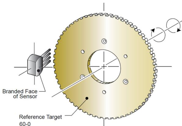
Figure 1: Magnetic Encoder Diagram
