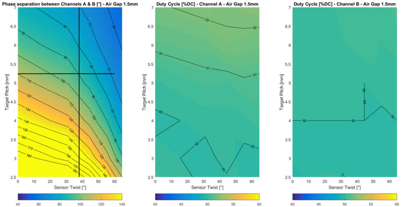
Figure 10: Sensor Twist over Target Pitch with Air Gap of 1.5 mm and Tooth/Pitch Ratio of 0.4
