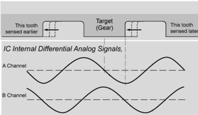
Figure 2: Differential Signals Sensed by the Sensor
