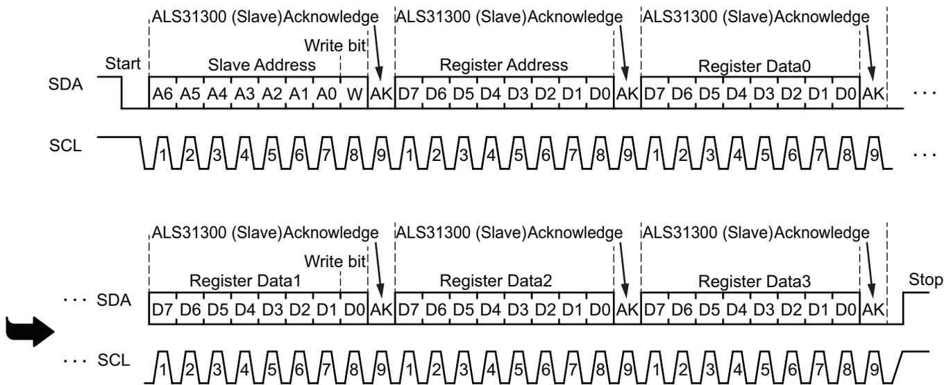
Figure 3: I<sup>2</sup>C Write Timing Diagram
