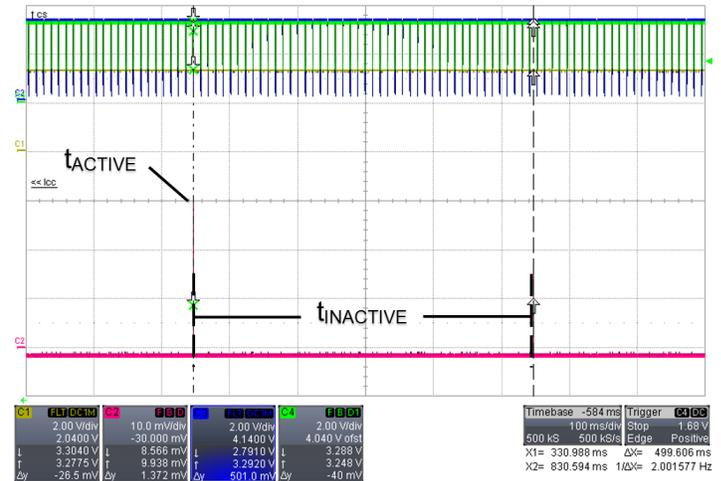
**Figure 8:  $I_{CC}$  Profile During LPDCM**
