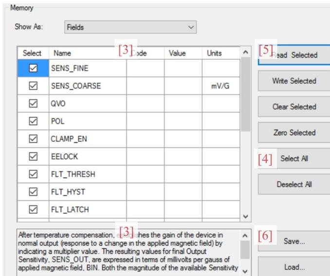
**Figure 3: Memory Panel from the A1365 Samples Programmer**
