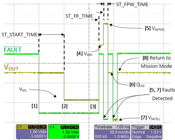
**Figure 6: Self-Test Mode Sequence**
