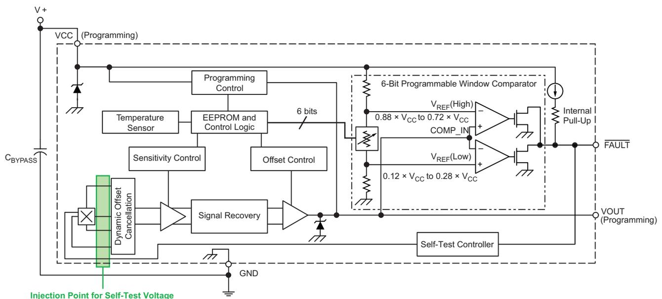
Figure 1: A1365 Functional Block Diagram
