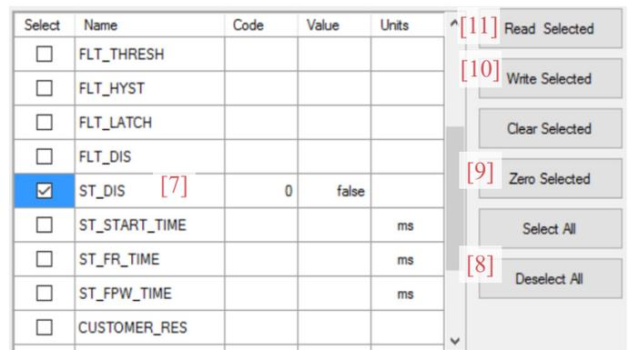
**Figure 4: Self-Test Enable from the A1365 Samples Programmer**
