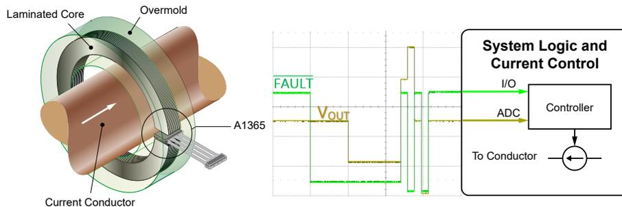
**Figure 8: Application Schematic with A1365, ADC, and Overcurrent Fault Control**
