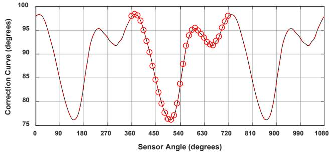
**Figure 21: Correction curve replicated three times, least-squares fit, central points used**
