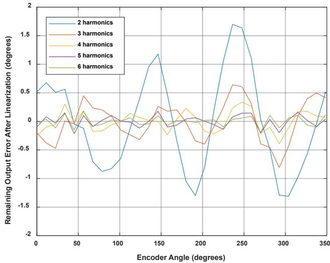
**Figure 19: Remaining angle error after linearization with an increasing amount of harmonics for the example in this document**
