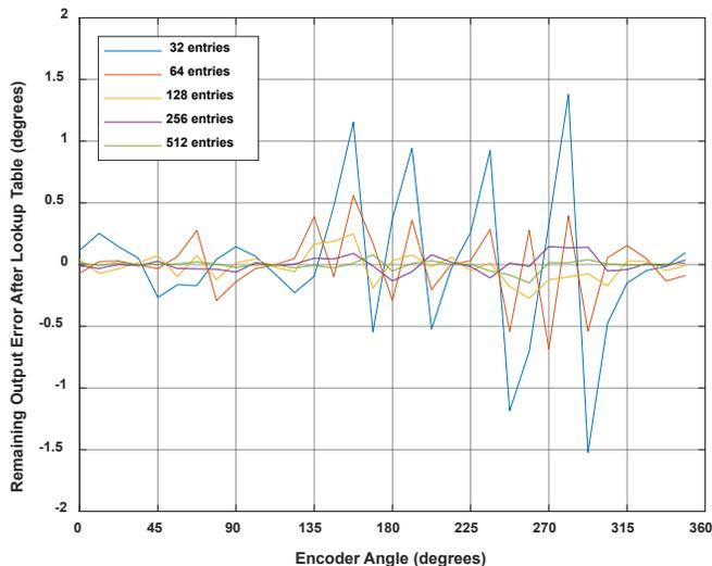
**Figure 24: Remaining angle error after linearization with an increasing amount of lookup table entries for the example in this document**
