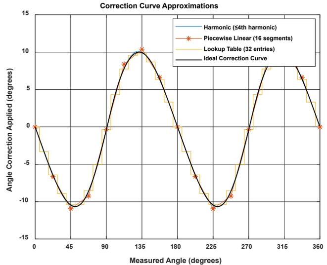
Figure 11: Correction curve (black) and three approximation methods
