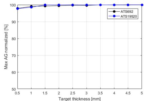
Figure 25: Normalized maximum air gap vs. target thickness.
