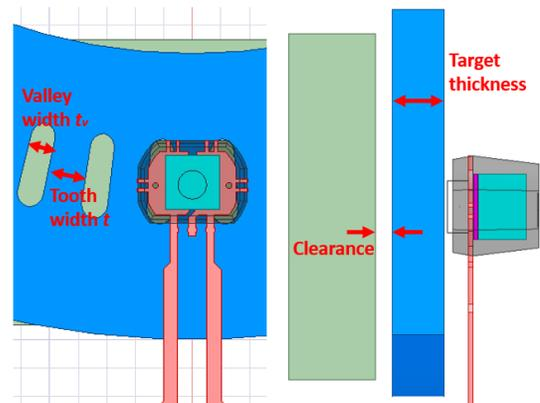
Figure 23: Definition of target thickness and valley clearance
