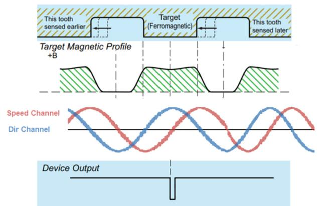
Figure 2: Output in the middle of the tooth
