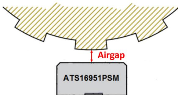
Figure 6: Air gap definition
