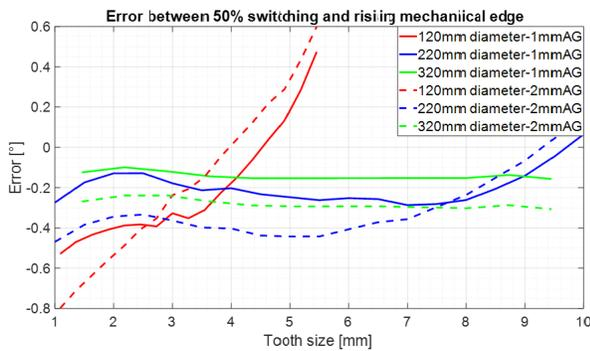
Figure 12: Dir channel rising edge error
