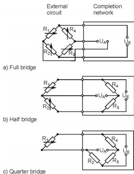
Figure 7: Possible bridge configuration of strain gauges
