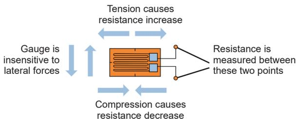
Figure 6: Resistance behavior of strained gauge
