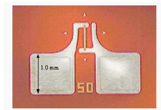
Figure 2: Vertical semiconductor strain gauge between metal pads.
