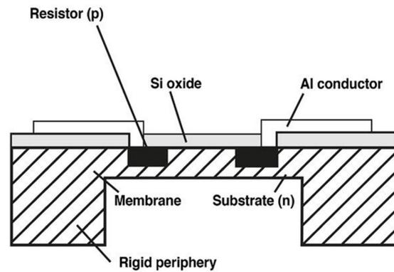
Figure 5: Semiconductor strain gauge
