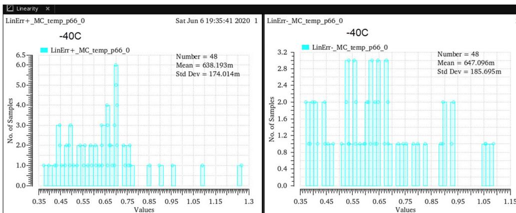
Figure 3: Histogram of linearity error at  $-40^{\circ}\text{C}$  for (starting with left) 0.667 mV/G positive currents and 0.667 mV/G positive currents.
