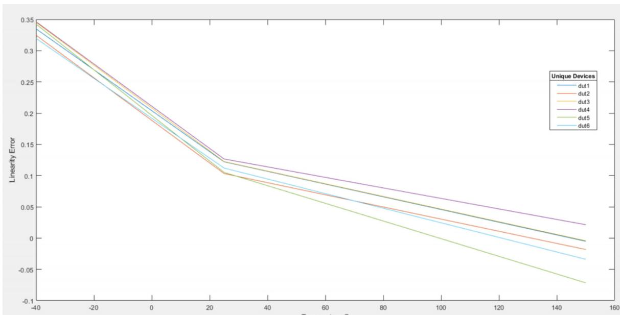
Figure 1: Measurement characterizing linearity error over temperature for six ACS70310 devices
