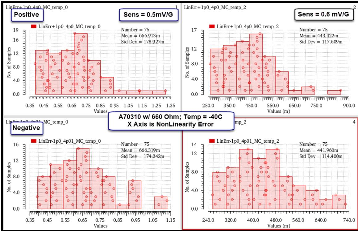
Figure 2: Histograms of linearity error at  $-40^{\circ}\text{C}$  for (starting with top left) 0.5 mV/G positive currents, 0.6 mV/G positive currents, 0.5 mV/G negative currents, and 0.6 mV/G negative currents.
