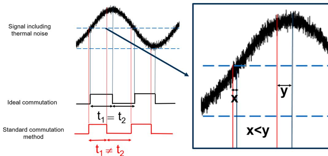
Figure 2: Threshold location effect on pulse position accuracy.
