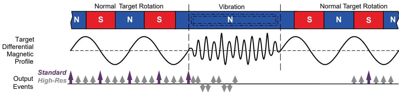
Figure 4: Vibration recovery using high resolution.
