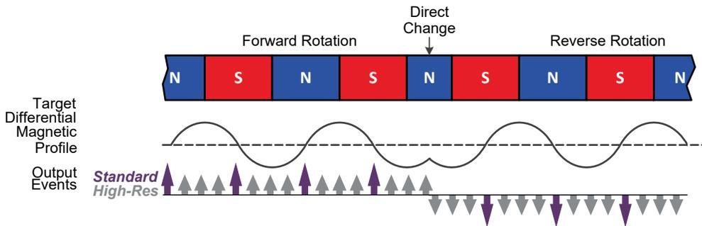
Figure 3: Direction change detection with high resolution.
