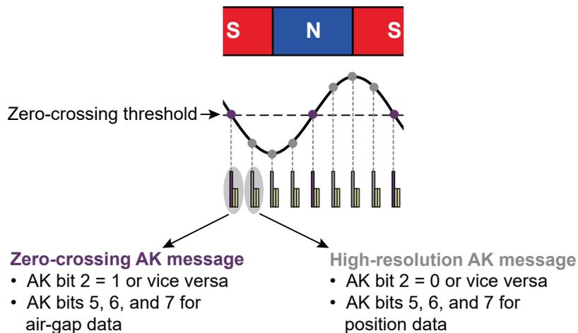
Figure 6: Distinction of high-resolution vs. standard pulses.
