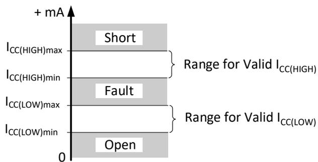
Figure 4: Two wire digital levels
