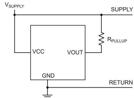
Figure 8: Conversion of three-wire to two-wire
