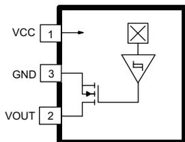
Figure 1: Example three-wire IC pinout
