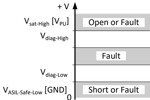
Figure 7: Three-wire output states including diagnostic
