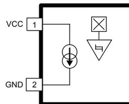
Figure 3: Example two-wire IC pinout
