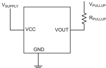
Figure 2: Three-wire interface circuit
