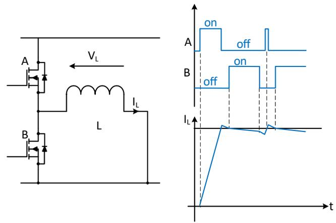
Figure 2: Complementary switching circuit.
