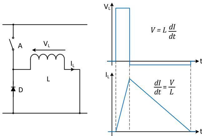
Figure 1: Driving inductive load.
