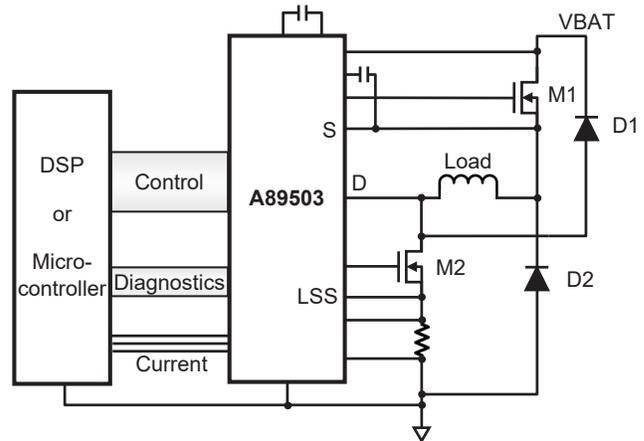
Figure 4: A89503 PWM load current control.
