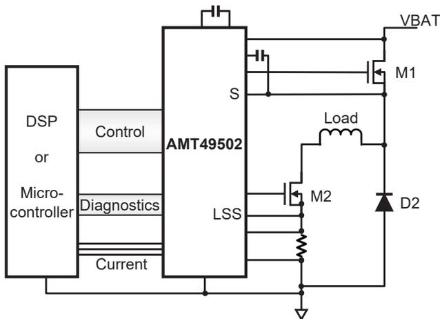
Figure 3: AMT49502 PWM load current control.
