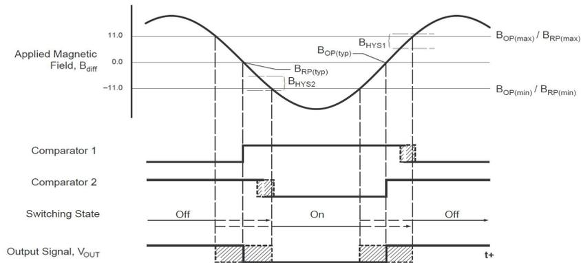
Figure 1: Example of switching scheme for a speed-only sensor
