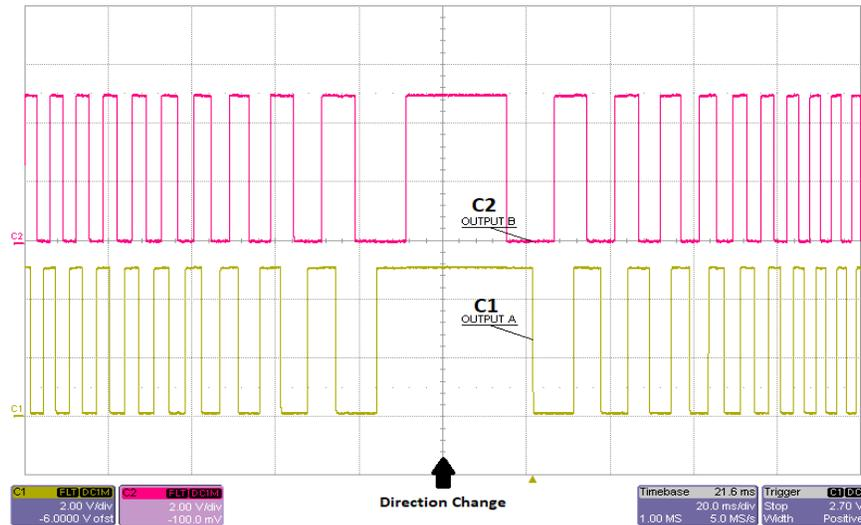
Figure 8: Scope capture of the A and B output signals (C1, C2) from the AB speed protocol during a direction change
