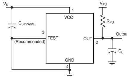
Figure 3: Typical application circuit for an open drain speed-only sensor. Bypass and load capacitors added to meet EMC requirements
