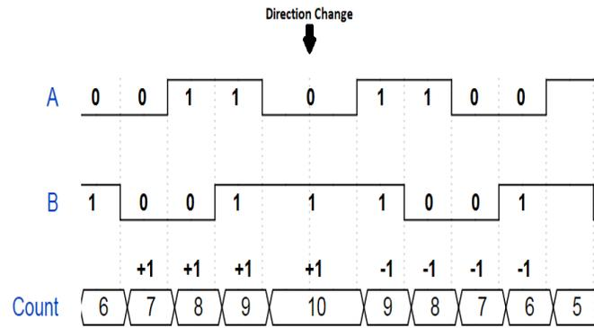
Figure 9: AB protocol encoding state transitions
