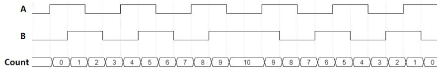
Figure 7: Incremental counting using the AB speed protocol
