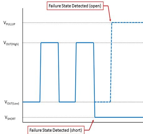
Figure 12: ECU Fault Condition detection
