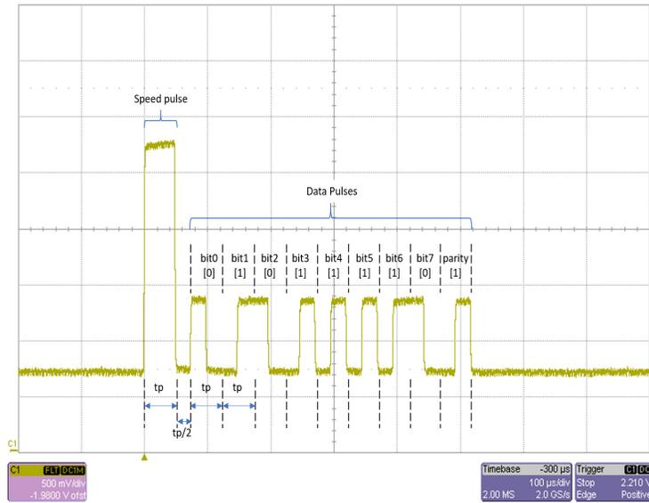
Figure 11: Scope capture of a single AK message showing a speed pulse followed by the data pulses and the decoding of the data pulses to bits
