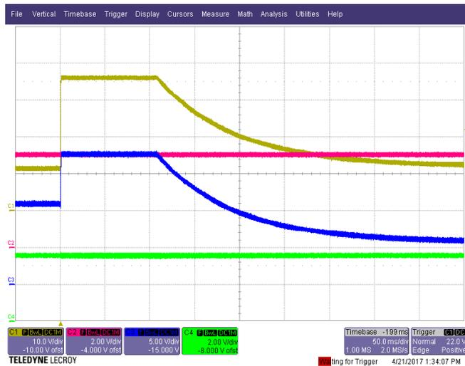
Figure 7: Transient waveforms during load-dump
