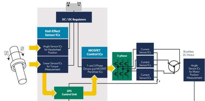
Figure 1: Typical applications of sensors in EPS applications
