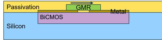
Figure 3: GMR sensor IC monolithic solution—Simplified layer cross section.
