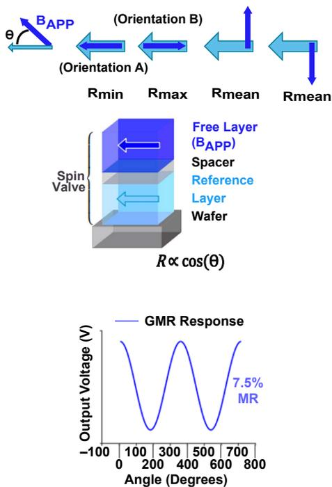
Figure 2. Simplified GMR structure and response to applied magnetic field orientation.
