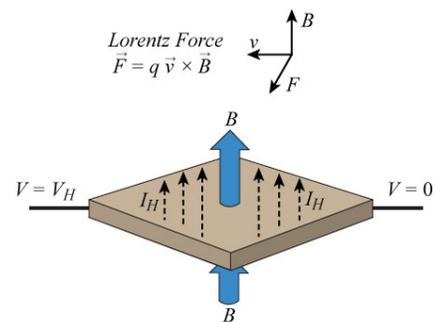
Figure 1: Simplified Hall plate diagram.
