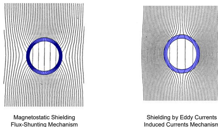
Figure 6: Flux Shunting and Eddy Currents
