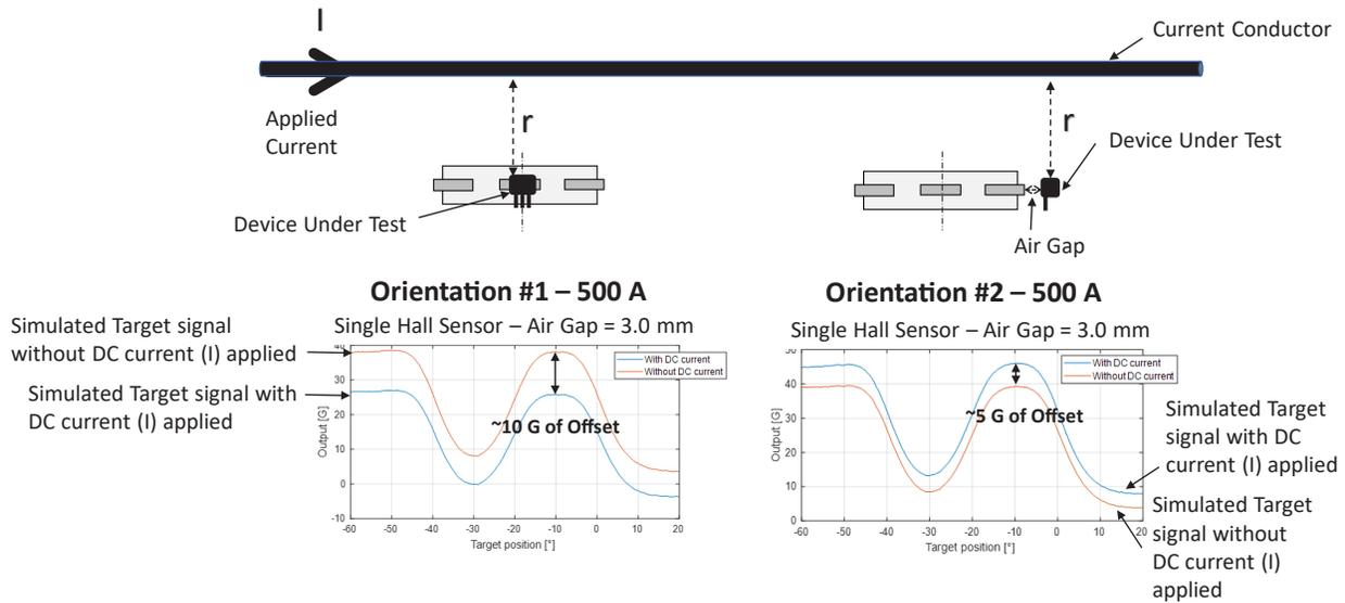
Figure 7: Impact of External Field Orientation to Single Hall Cam Sensor (ATS16301PSL)
