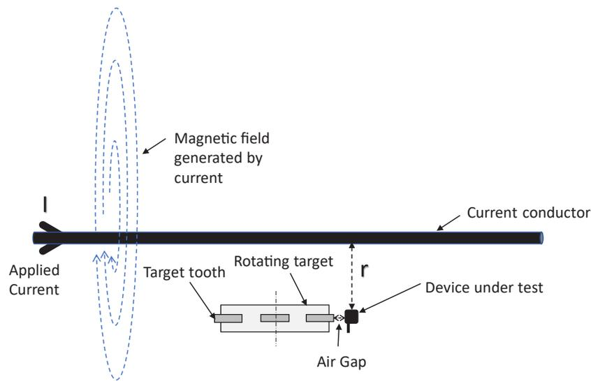
Figure 4: Single Current Wire Test
