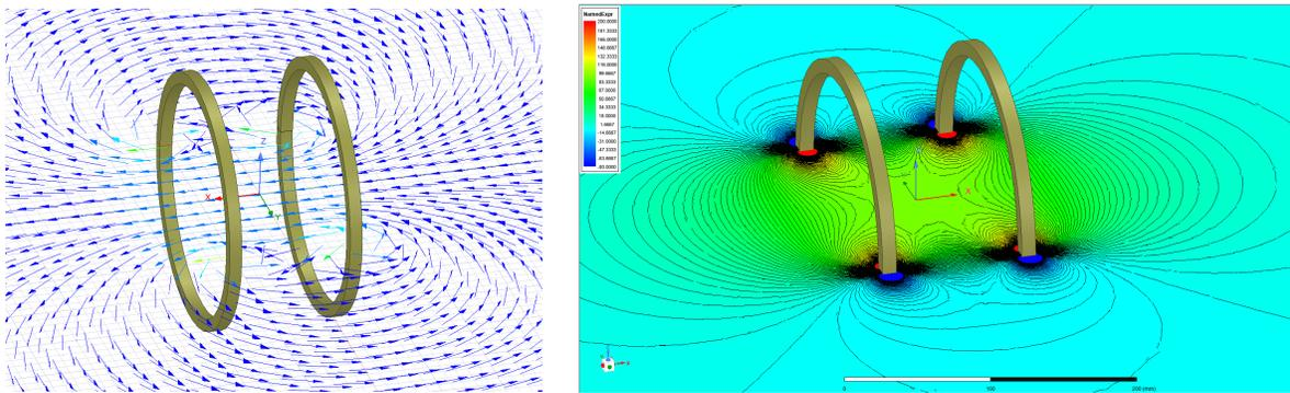
Figure 5: Helmholtz Coil Generating Large Homogeneous Field Area
