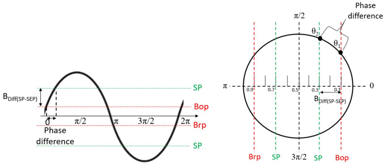
Figure 7: Sine wave (left) and phasor (right) representation of the differential signal.  $B_{OP}$  (red),  $B_{RP}$  (red) and  $SP$  (green) thresholds respectively represent rising, falling switch point, separation of 20%. In this figure,  $B_{OP}$  and  $B_{RP}$  are set to 60% and 40%. Other switch points may be used depending on the sensor of interest and are specified on the datasheet.
