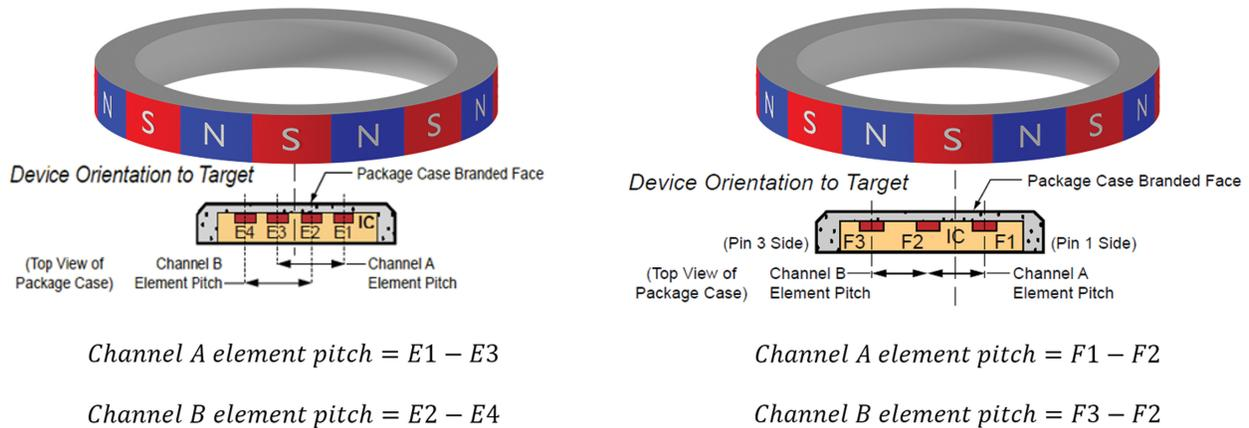
Figure 2: Element pitch representation for GMR (left) and Hall (right) speed and direction sensors
