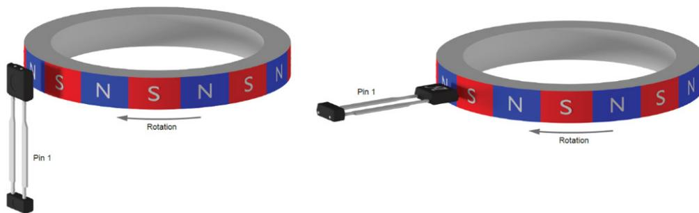
Figure 3: Magnetic field orientation on Allegro Hall based (left only) and GMR (left and right sensor installation) speed sensor
