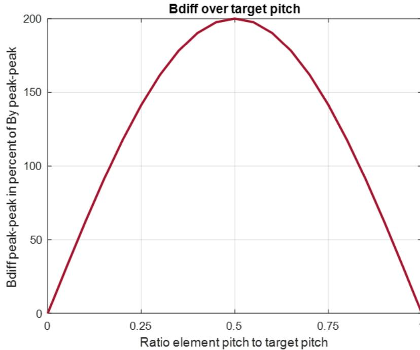
Figure 4: Influence of element pitch to target pitch ratio on differential signal amplitude
