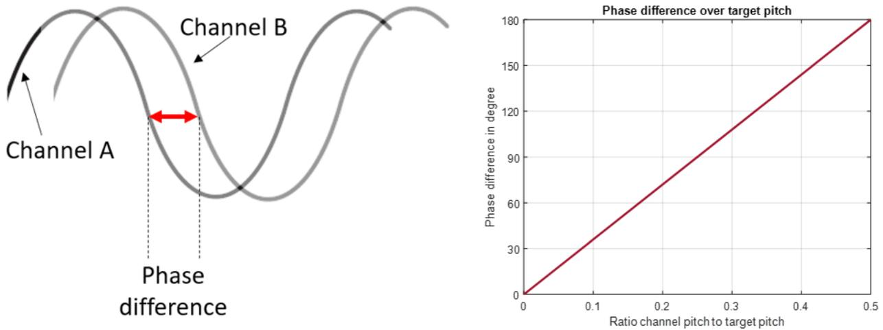
Figure 5: Impact of channel pitch to target pitch ratio on phase difference between differential signals
