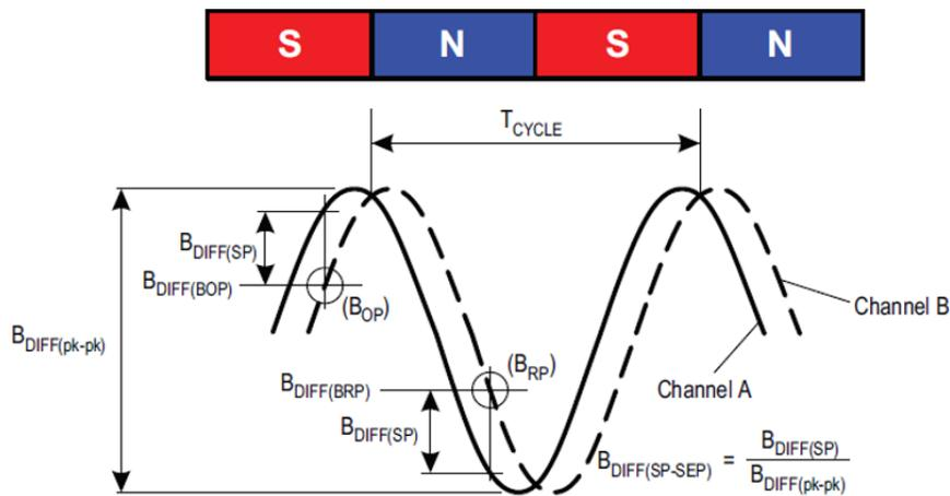
Figure 6: Definition of switch point separation. Bop and Brp represent respectively rising and falling switch points.
