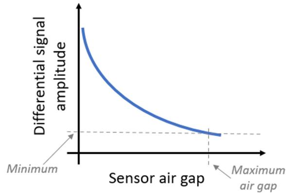
Figure 8: Maximum air gap determination using target mapping
