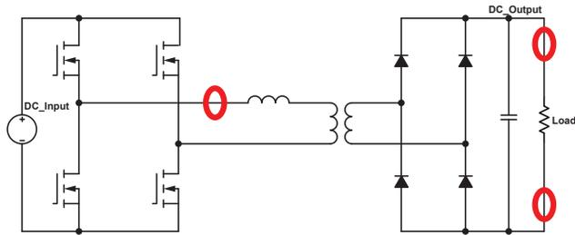
Figure 3: Resonant DC-DC converter circuit. Red circles show current sensing locations. Sensor on the left is for the input current and requires isolation. Current sensors on the right are for output current located either on the low or high side depending on selected approach.
