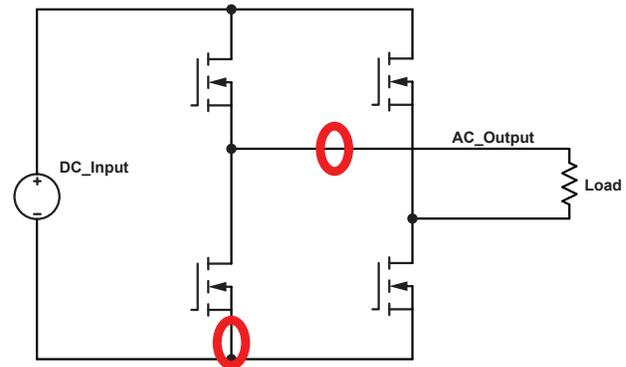
Figure 4: Single-phase inverter circuit. Red circles show current sensing locations. One circle represents in phase sensing, before the load, while the other represents low side sensing where the sensor is placed between the load and ground.
