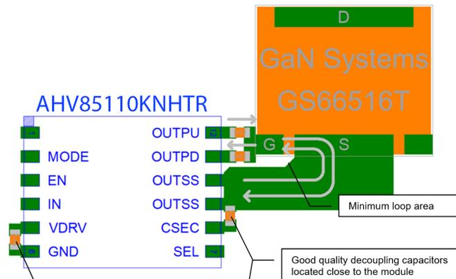
Figure 2: AHV85110KNHTR PCB layout with GaN Systems GS66516T
