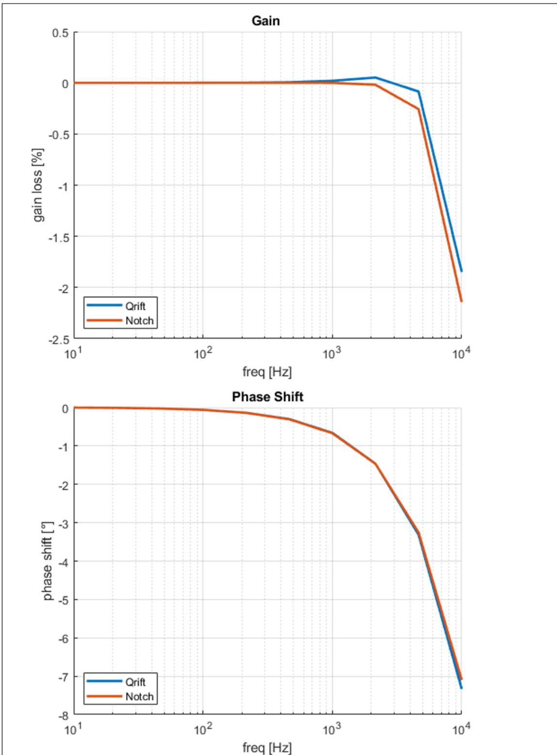
Figure 4: Frequency response of Notch (red) and Q-Rift(blue) PCB for AC applications.
