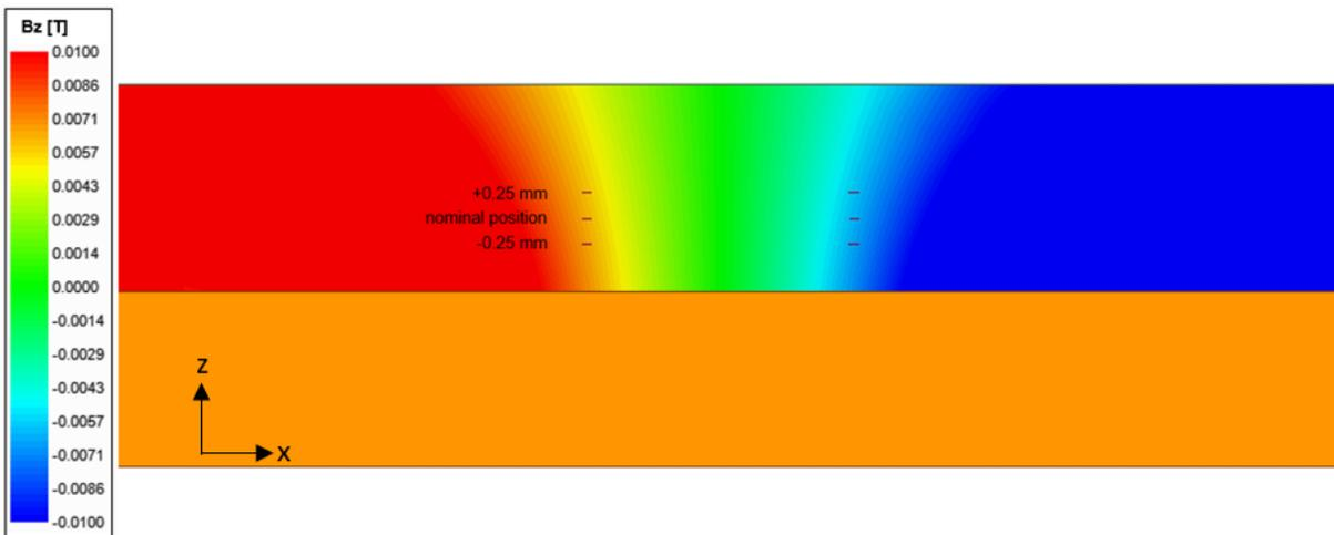
Figure 2: Bz-Field for a notch width of 8 mm. The scale is cut to  $\pm 0.01$  T to show the Bz gradient at the Hall plate locations.
