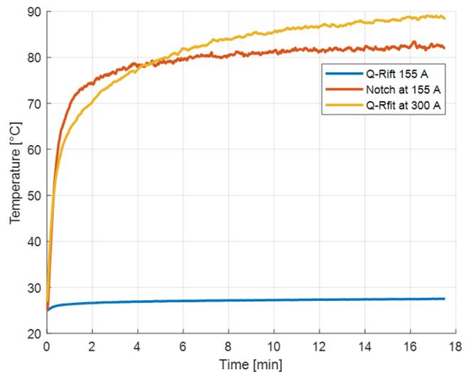
Figure 7: PCB Temperature over time after applying 155 and 300 A, respectively.
