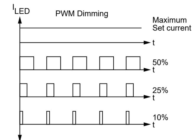
Figure 3: PWM Dimming
