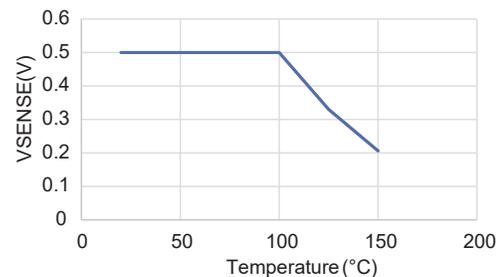
Figure 10:  $V_{SENSE}$  vs. Temperature
