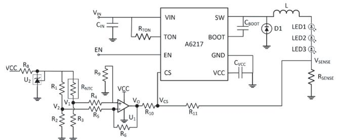
Figure 14: A6217 Buck LED Driver and Op-Amp with LDO for Derating Proportional to Temperature
