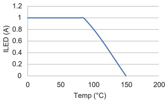
Figure 13: A6217 Thermal Derating,  $I_{OUT}$  vs. Temperature
