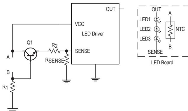
Figure 11: LED Driver with Transistor in Emitter-Follower Configuration and
