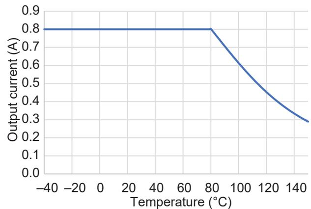
Figure 15: A6217 Temperature vs. Output Current
