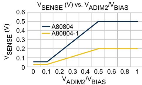
Figure 8: A80804 SENSE Voltage vs. ADIM and BIAS Ratio
