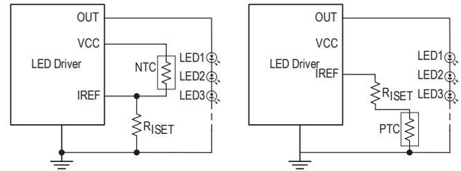
Figure 4: Combinations for Thermistor and  $R_{ISET}$  for Derating
