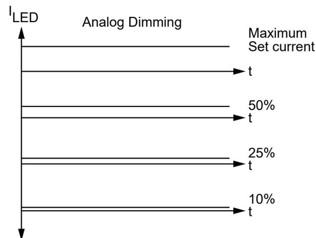
Figure 2: Analog Dimming
