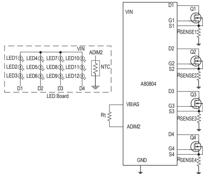
Figure 9: A80804 Thermal Derating Using Analog Dimming
