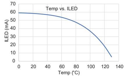
Figure 6: Temperature vs.  $I_{LED}$
