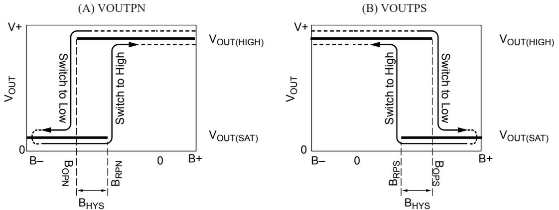
Figure 2. Operation with Unipolar Mode Selected (SELECT Pin Grounded)
