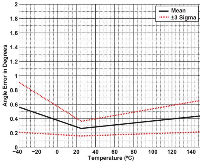
Figure 22: Peak Angle Error over Temperature (300 G)
