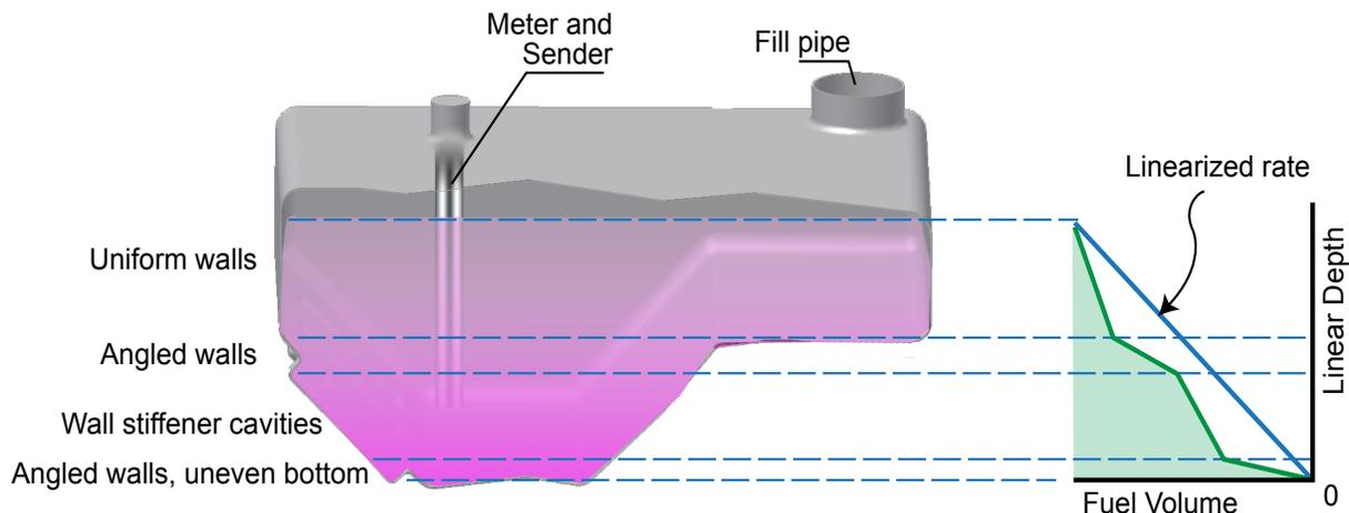
**Figure 18:** An integrated vehicle fuel tank has varying volumes according to depth due to structural elements. As shown in the chart, this results in a variable rate of fuel level change, depending on volume at the given depth, and a linearized transfer function can be used against the integral volume.
