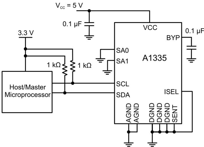
(A) Typical A1335 configuration using I<sup>2</sup>C interface; A1335 set up for serial address 0xC
