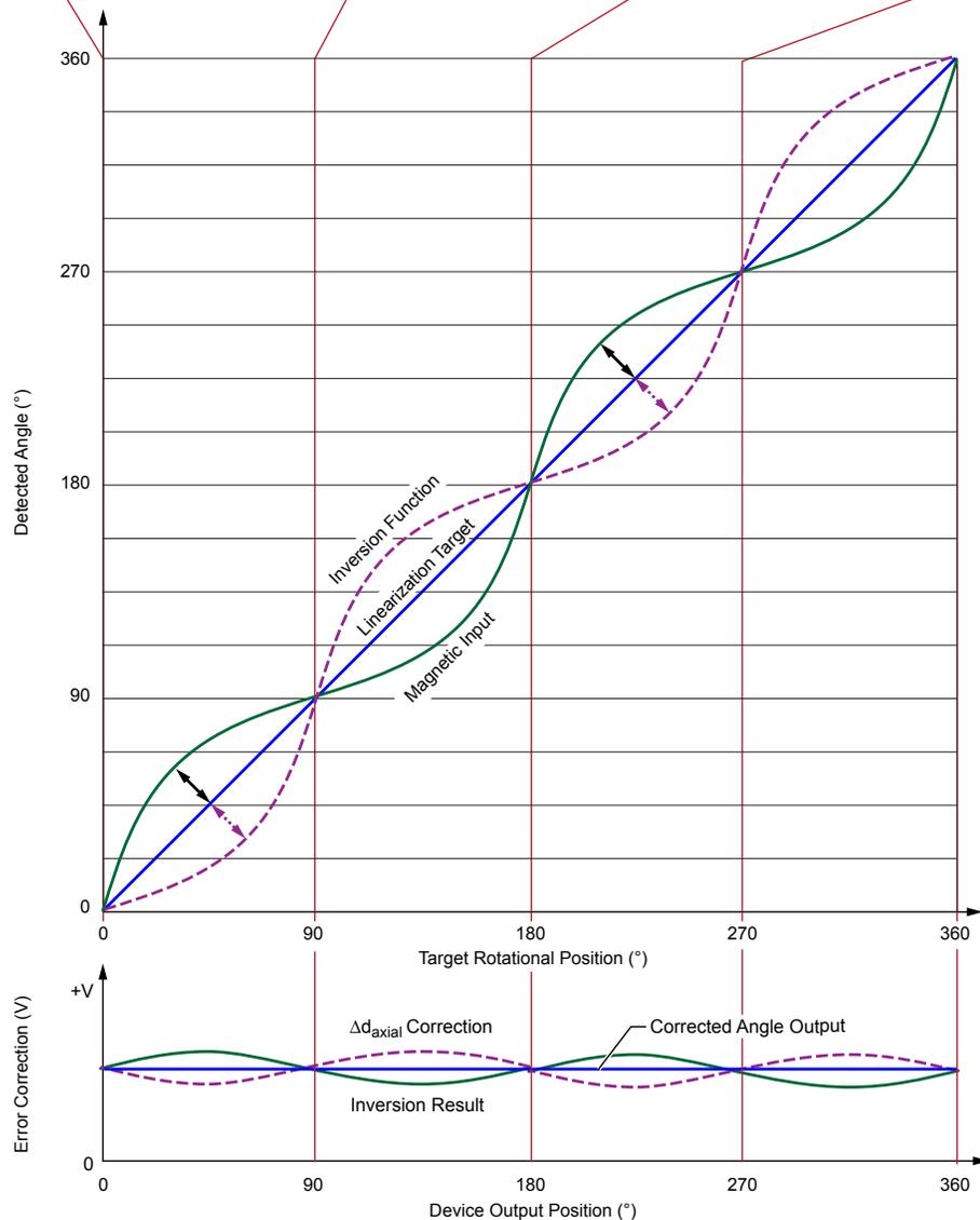
Figure 19b: Any eccentricity is evaluated as an error. Systematic eccentricity can be factored out by appropriate linearization coefficients. For off-axis applications, the harmonic linearization method is recommended.
