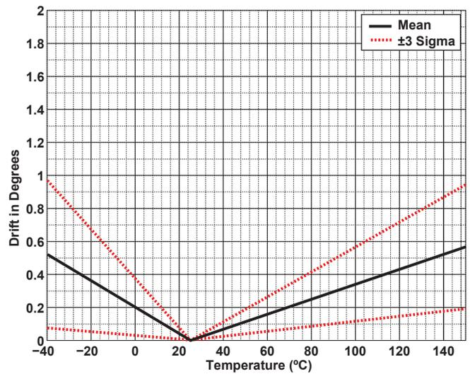
Figure 23: Maximum Temperature-Induced Drift from 25°C (300 G)
