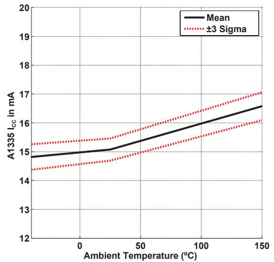
Figure 27: I<sub>CC</sub> over Temperature
