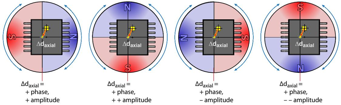
Figure 19a: With the axis of rotation aligned with the Hall element, linearization coefficients are a simple inversion of the input.
