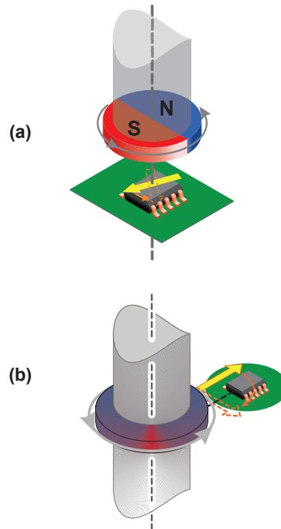
Figure 13: Typical On-Axis (a) and Off-Axis (b) Orientation
