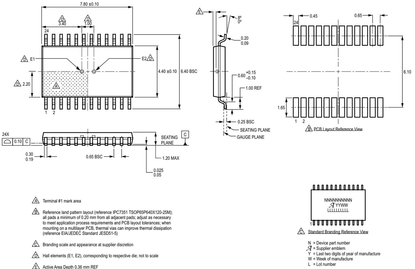
Figure 29: Package LE, 24-Pin TSSOP (Dual-Die Version)
