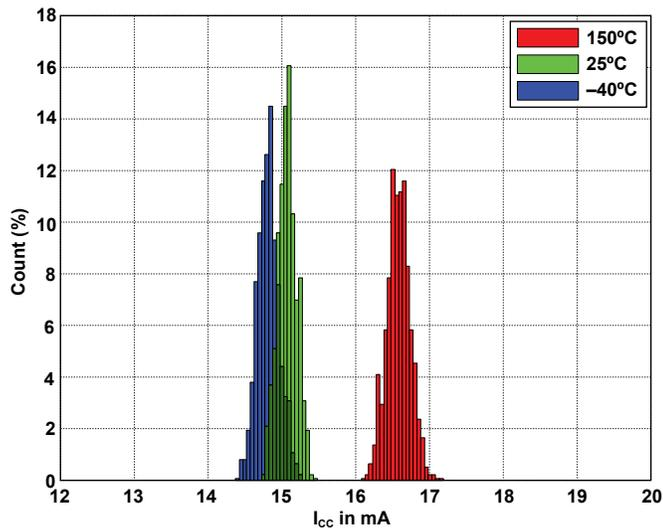
Figure 26: I<sub>CC</sub> Distribution over Temperature
