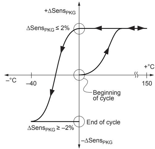
**Figure 7: Package Hysteresis Sensitivity Drift During Temperature Cycling**
