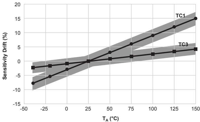
**Figure 6: Sensitivity Drift Through Temperature Range ( $\Delta Sens_{TC}$ )**
