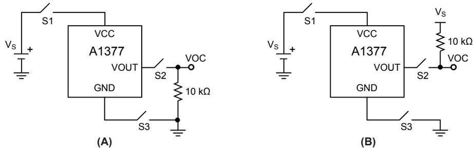
**Figure 9: Diagnostic Application Circuits: (A) Pull-Down, (B) Pull-Up**
