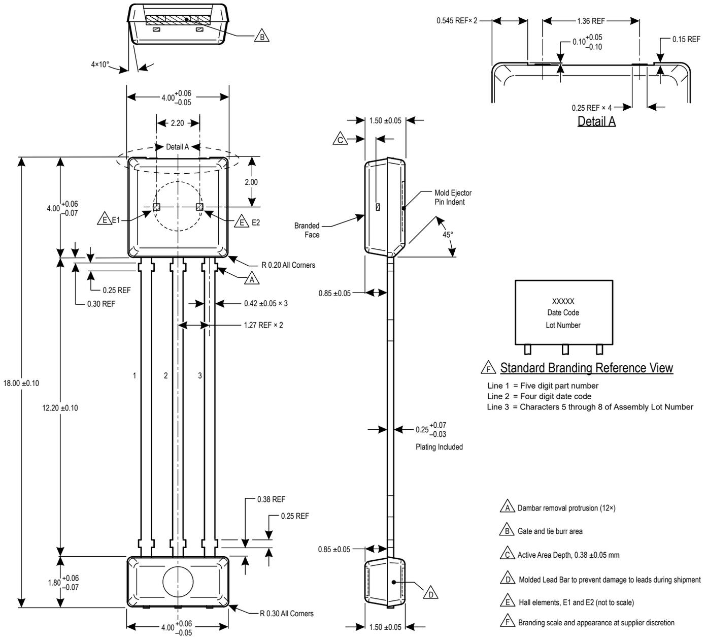
Figure 7: Package UC, 3-Pin SIP
