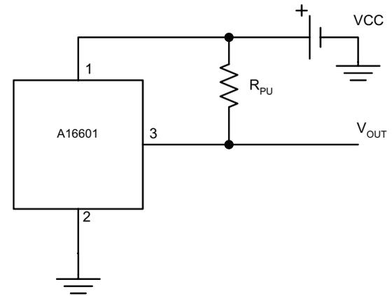
**Figure 6: Basic application circuit. A pull-up resistor, R<sub>PU</sub>, is required with the output driver.**
