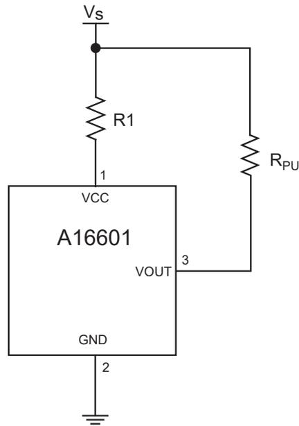
Figure 3: Recommended EMC Test Circuit
