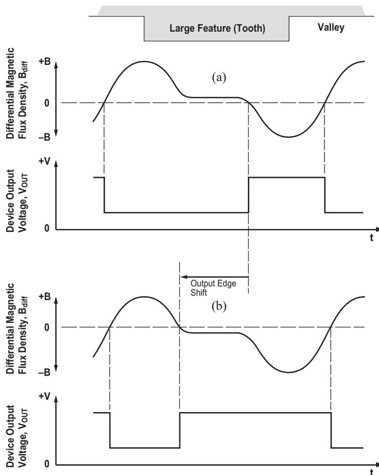
**Figure 5: Large Feature Effects. (a) Large target feature but no device offset, normal edge position. (b) Large target feature with negative device offset, shifted (advanced) output edge position.**
