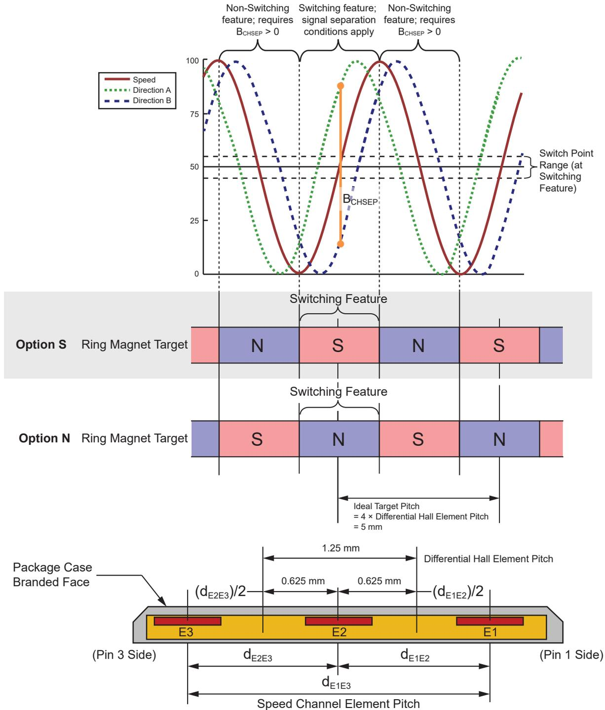
Figure 10: Channel Separation and Signal Inversion Definitions
