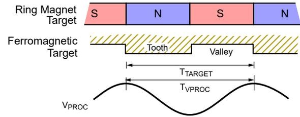
$V_{PROC}$  = the processed analog signal of the sinusoidal magnetic input (per channel)
