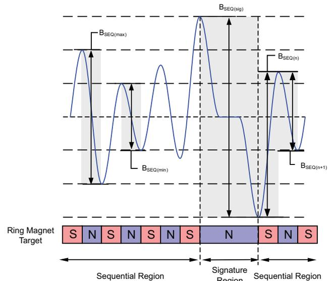
Figure 6: Differential Signature Amplification and Sequential Signal Variation
