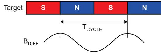
$B_{DIFF}$  = Differential Input Signal; the differential magnetic flux sensed by the sensor
