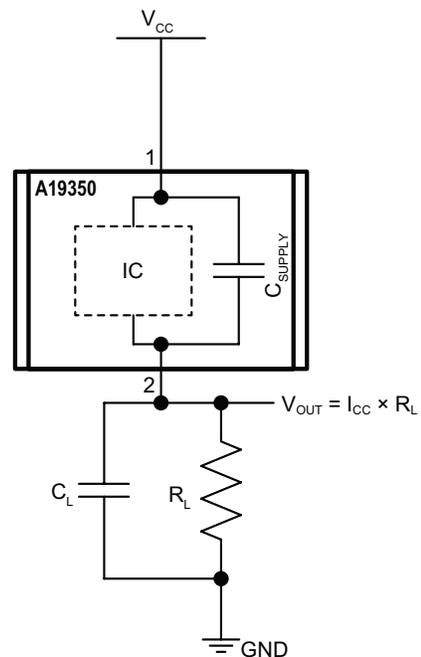
Figure 2: Application Circuit
