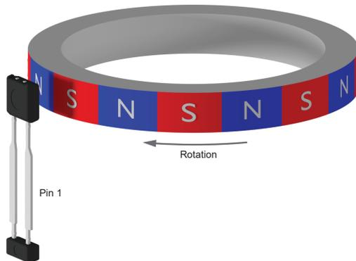
Figure 8: Parallel Orientation
