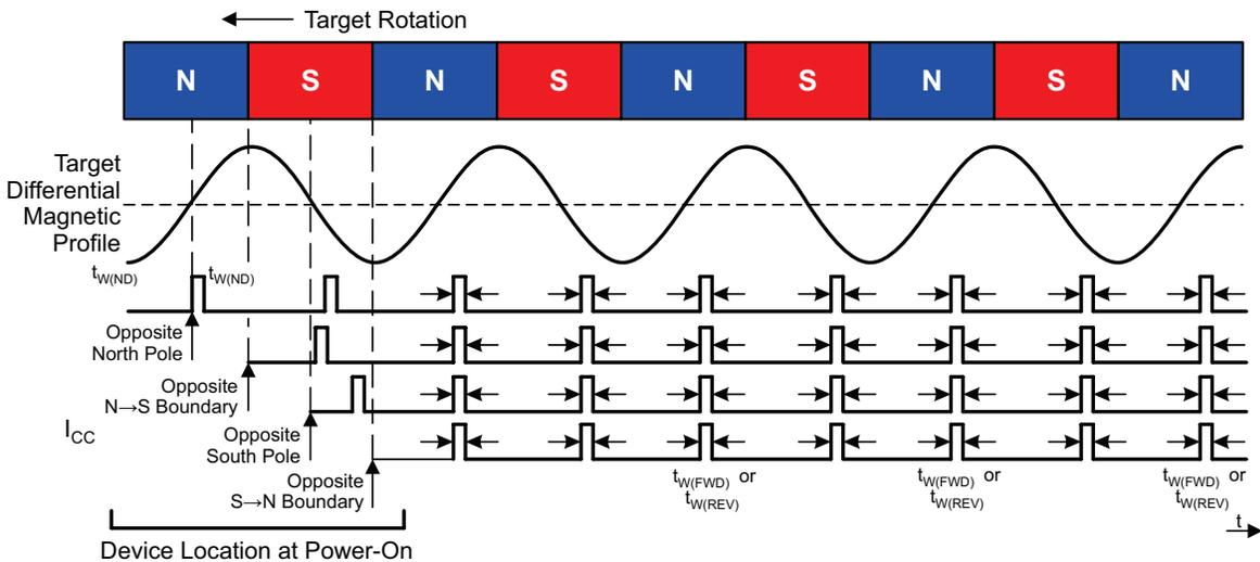
**Figure 12: Calibration Behavior of the -xPx Variant**
