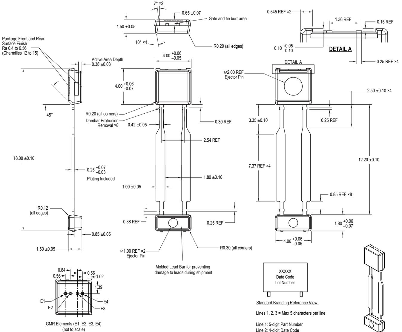
Figure 17: Package UB, 2-Pin SIP
