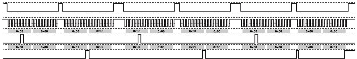
If an access violation occurs (address not unlocked), the transaction terminates, the corresponding RDN or WDN bit is set, and the XEE warning bit is asserted. The XEE bit in the ERR register also sets if the EEPROM write aborts.
