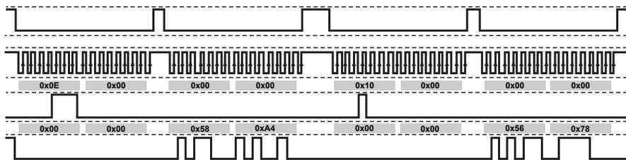
NOTE: It is possible to pipeline transactions in this example, i.e., send a new command while reading return data from the old command. Pipelining would result in 5 SPI frames to perform the transaction instead of 8.
