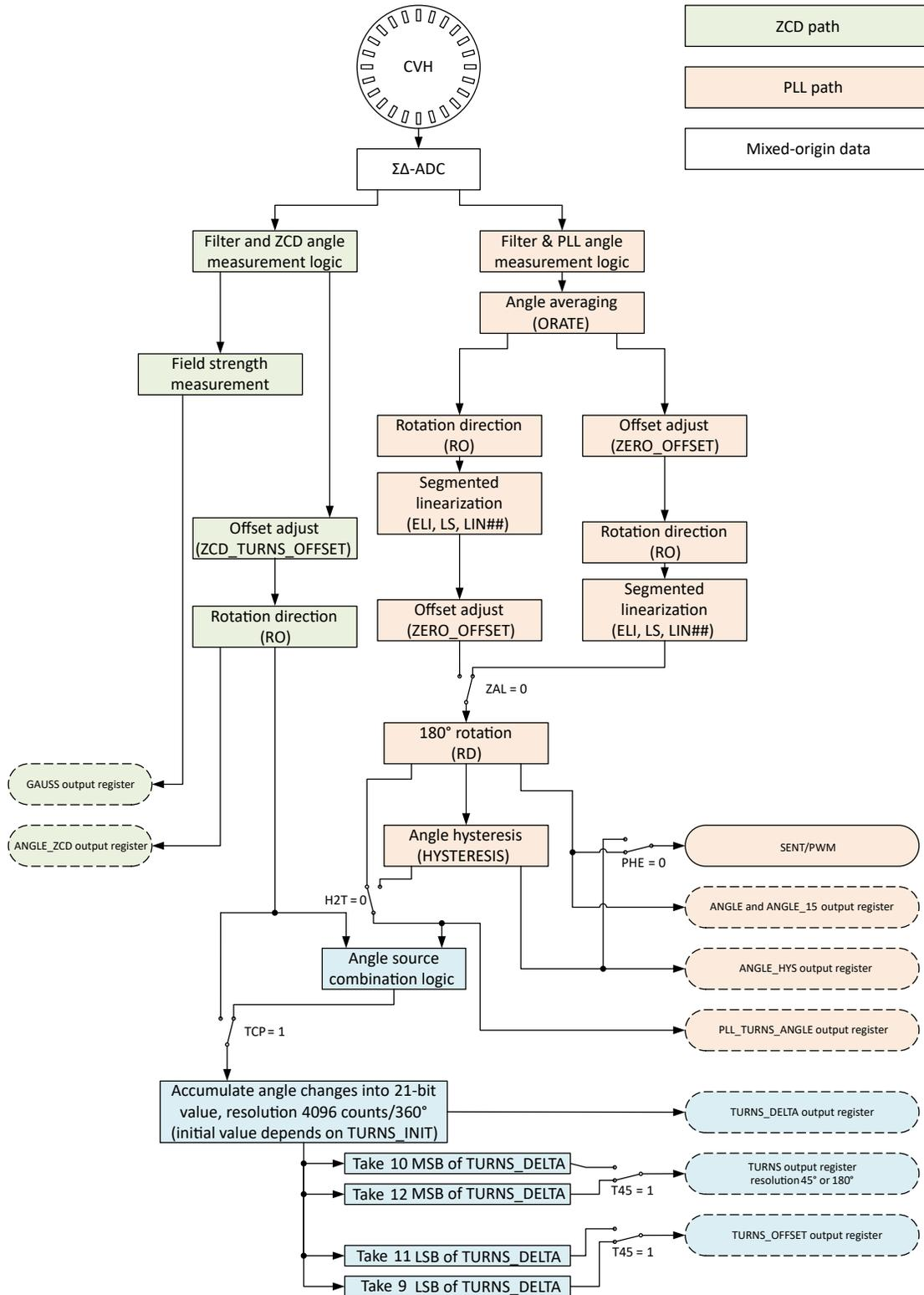
Figure 6: Angle Measurement – Sensor Readout Steps
