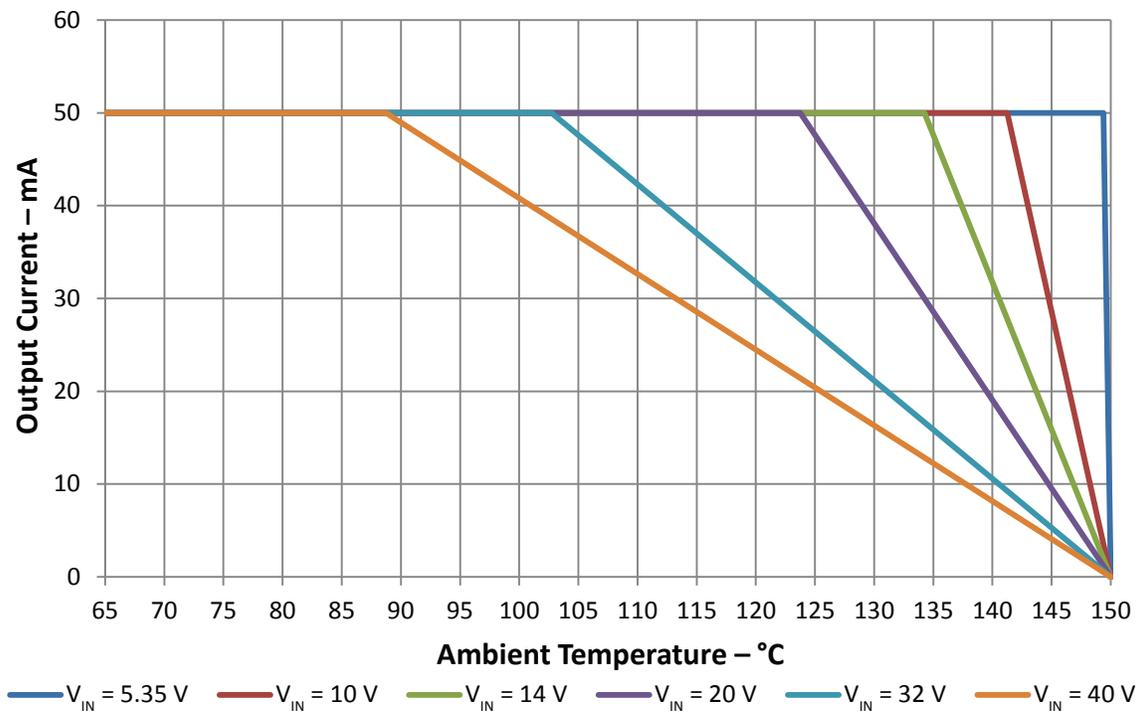
Figure 2: Output Current De-Rating vs. Input Voltage
