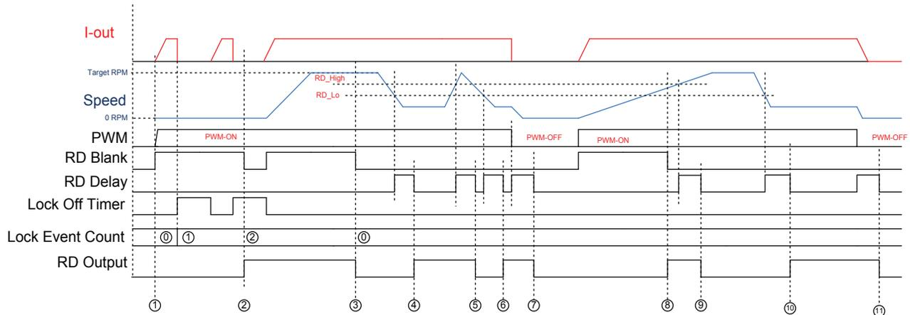
**Figure 6: RD Timing Diagram (LOCKEVT = 1)**
