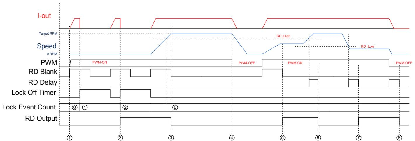
**Figure 4: RD Timing Diagram (LOCKEVT = 0)**
