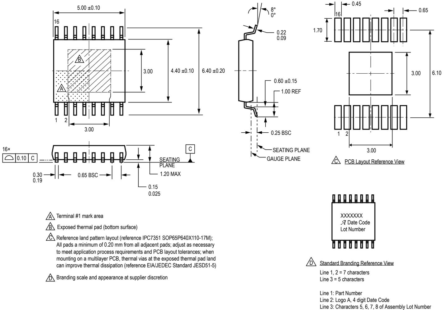
Figure 16: Package LP, 16-Lead TSSOP with Exposed Pad
