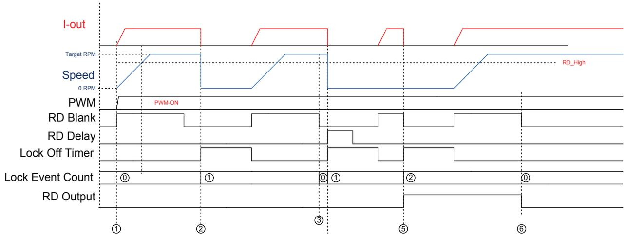
Figure 5: RD Timing Diagram (LOCKEVT = 0); lock condition while running
