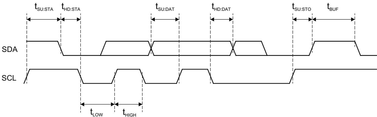
Figure 10: I<sup>2</sup>C-Compatible Timing Requirements
