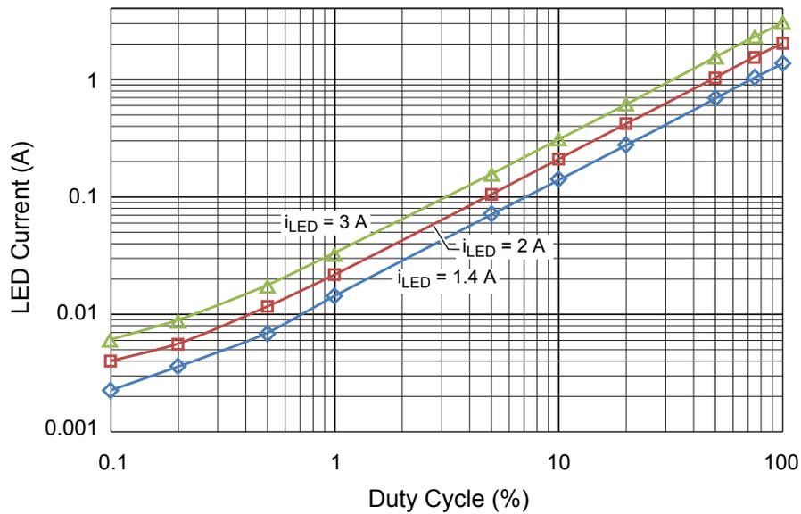
**Figure 5: Average LED Current versus PWM dimming percentage**
