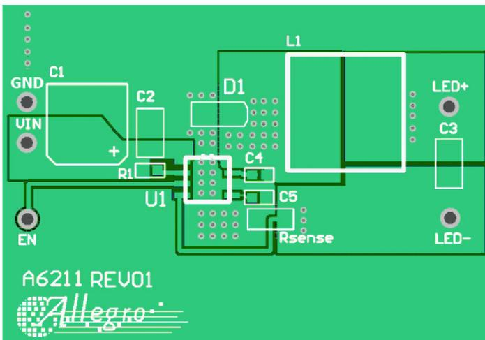
Figure 19: Example Layout for the A6211 Evaluation Board
