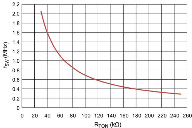
**Figure 6: Switching Frequency versus R<sub>TON</sub> Resistance**
