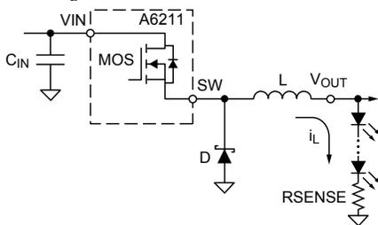
$$t_{ON} = k \times (R_{ON} + R_{INT}) \times (V_{OUT} / V_{IN})$$
