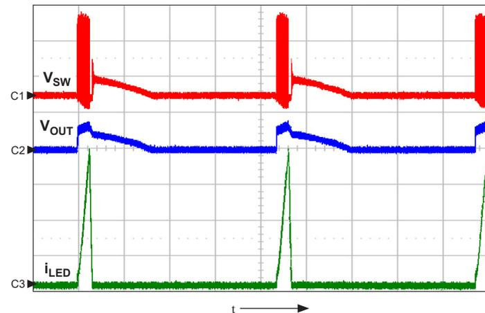
**Figure 10: A6211 overcurrent protection tripped in the case of a fault caused by the sense resistor pin shorted to ground; shows switch node,  $V_{SW}$  (ch1, 10 V/div.), output voltage,  $V_{OUT}$  (ch2, 10 V/div.), LED current,  $i_{LED}$  (ch3, 1 A/div.),  $t = 100 \mu$ s/div.**
