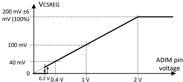
**Figure 7: ADIM Pin Voltage Controls SENSE Reference Voltage (hence LED current)**
