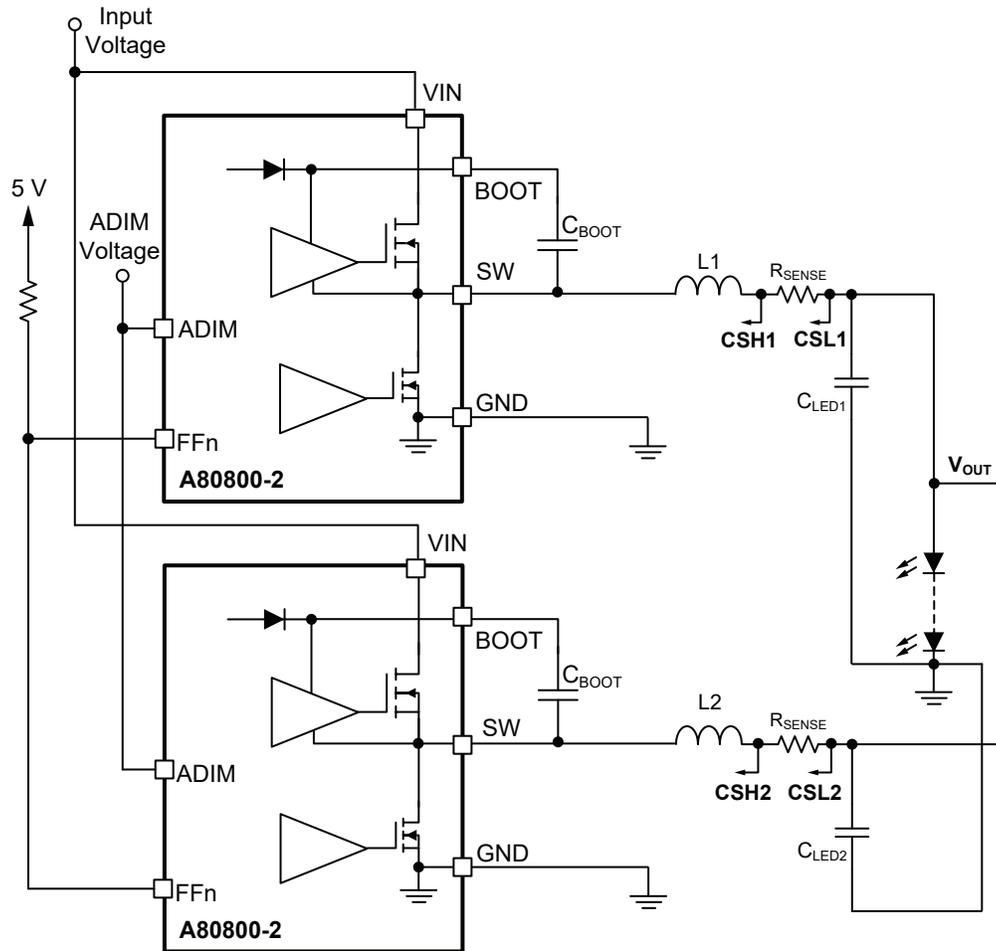
**Figure 19: Using 2 (or more) A80800-2 in parallel to drive the same LED string.
