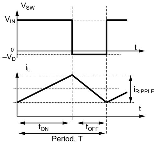
Note:  $V_D = R_{DSON(LS)} \times I_L$
