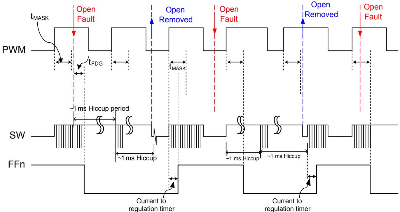
Figure 13b: LED Open Fault Timing Diagram Overview
