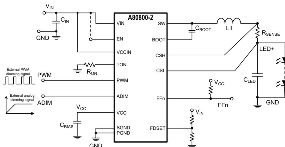
Figure 1: A80800-2 Typical Application Circuit
