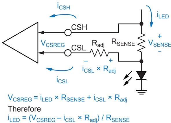
**Figure 3: How To Fine-Tune LED Current Using  $R_{adj}$**
