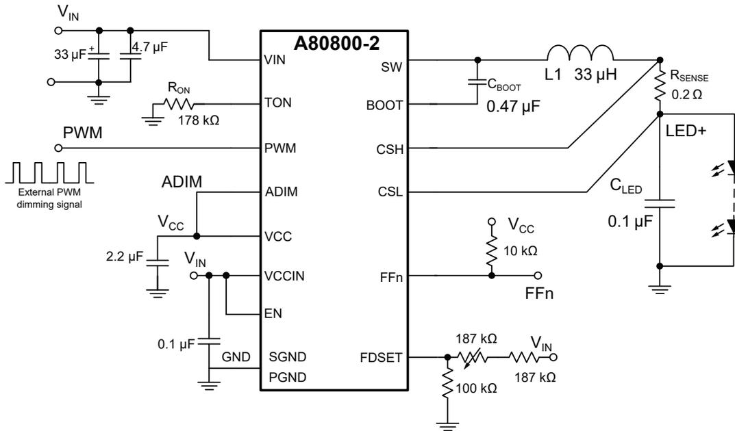
Figure 18: Application Circuit Example for A80800-2
