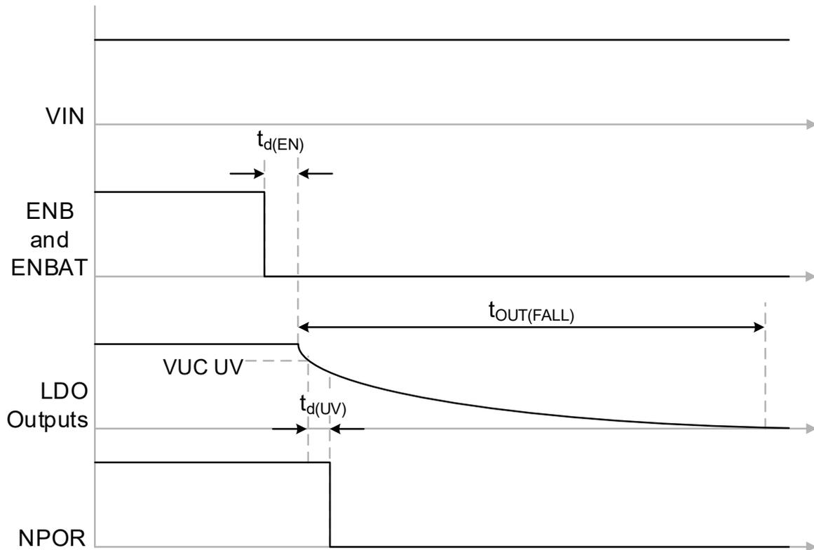
All LDO outputs start to decay  $t_{d(EN)}$  seconds after ENB and ENBAT are low. The time for an output to decay to zero,  $t_{OUT(FALL)}$ , varies for each LDO and depends on load and output capacitance. NPOR transitions low after VUC crosses its UV threshold
