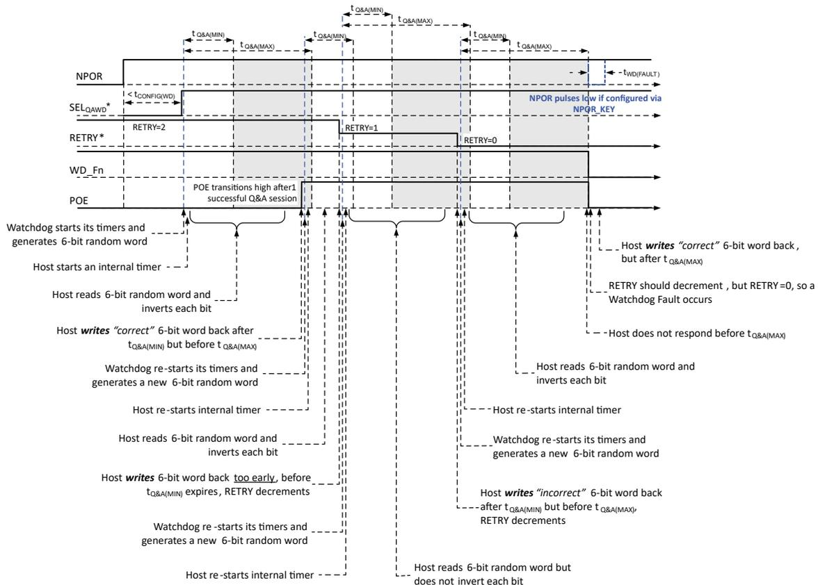
Figure 11: Q&A Selection, Operation, and Fault Examples.
