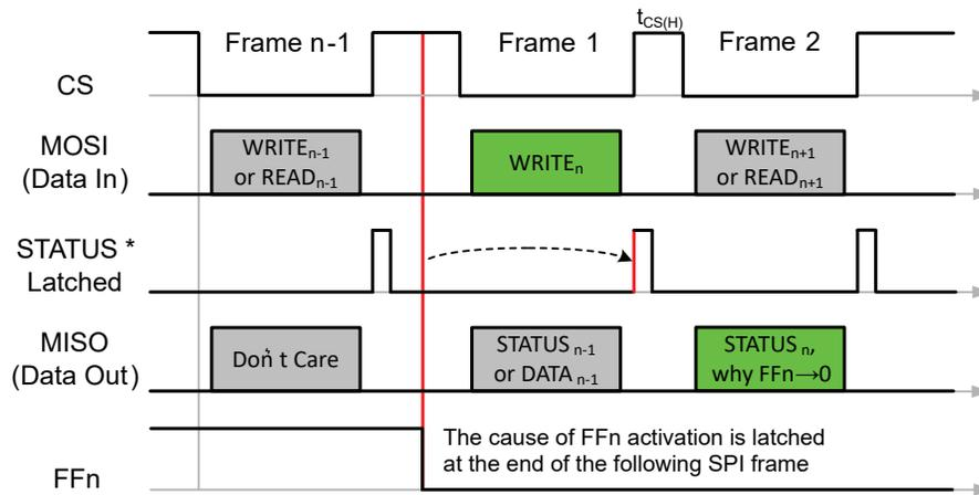
**Figure 16: Recommended SPI Operations after FF<sub>n</sub>→0**
