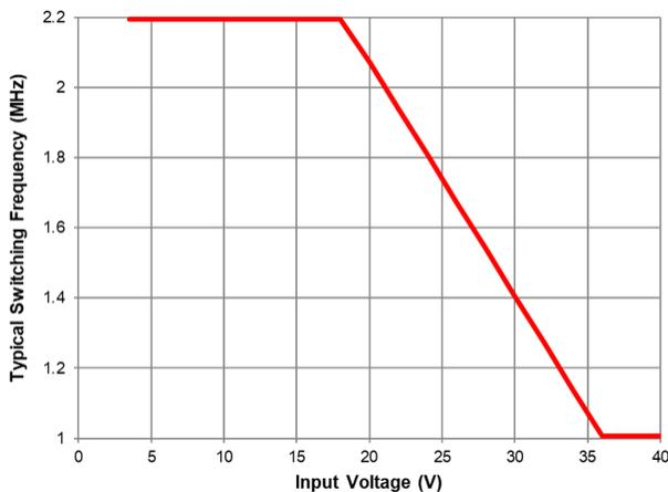
**Figure 17: Typical Switching Frequency versus Input Voltage**
