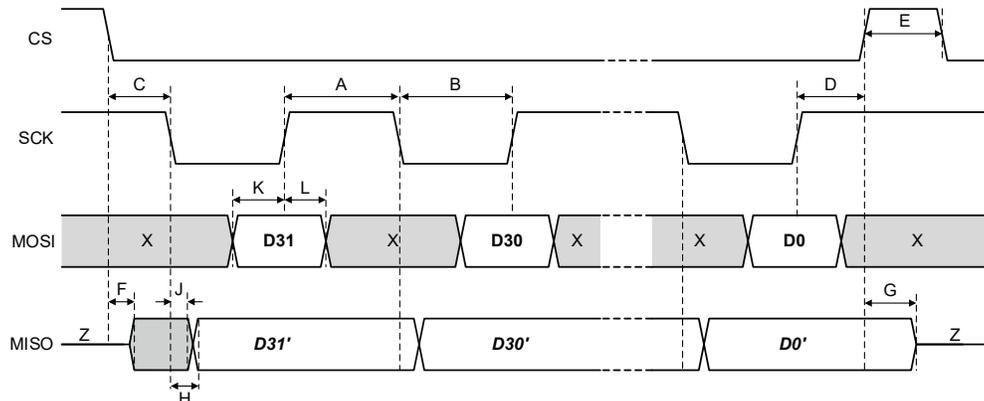
**Figure 1: Serial Interface Timing for Write and Read Cycles**
