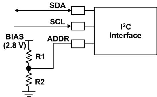
**Figure 2: Select I<sup>2</sup>C Address by Using Resistor Divider at ADDR Pin**
