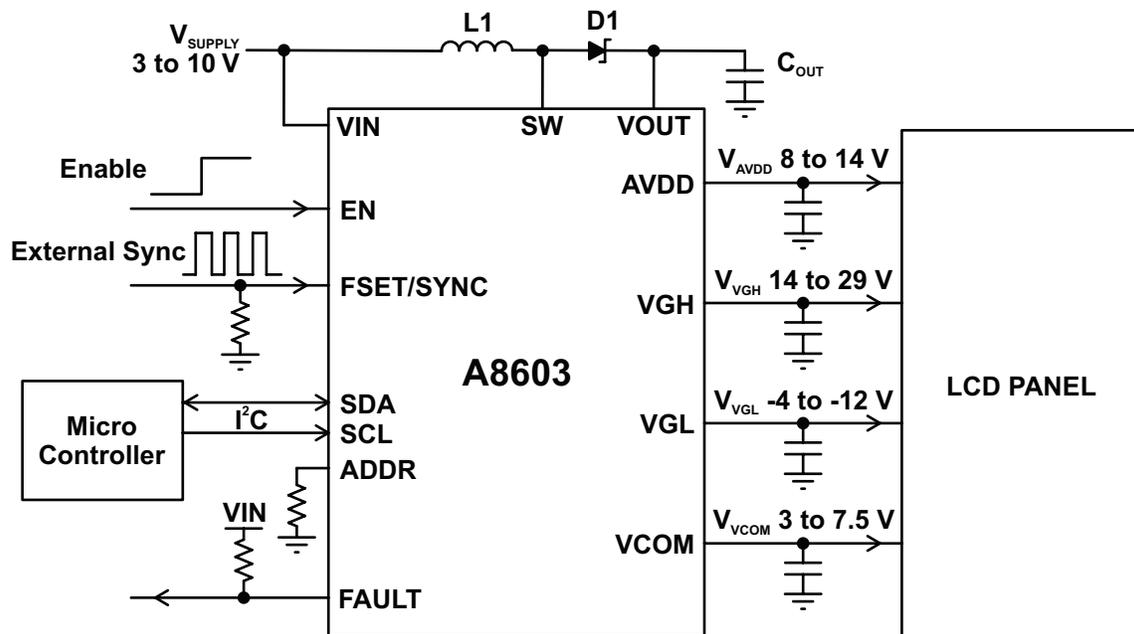
System Block Diagram Showing Typical Regulator Voltages
