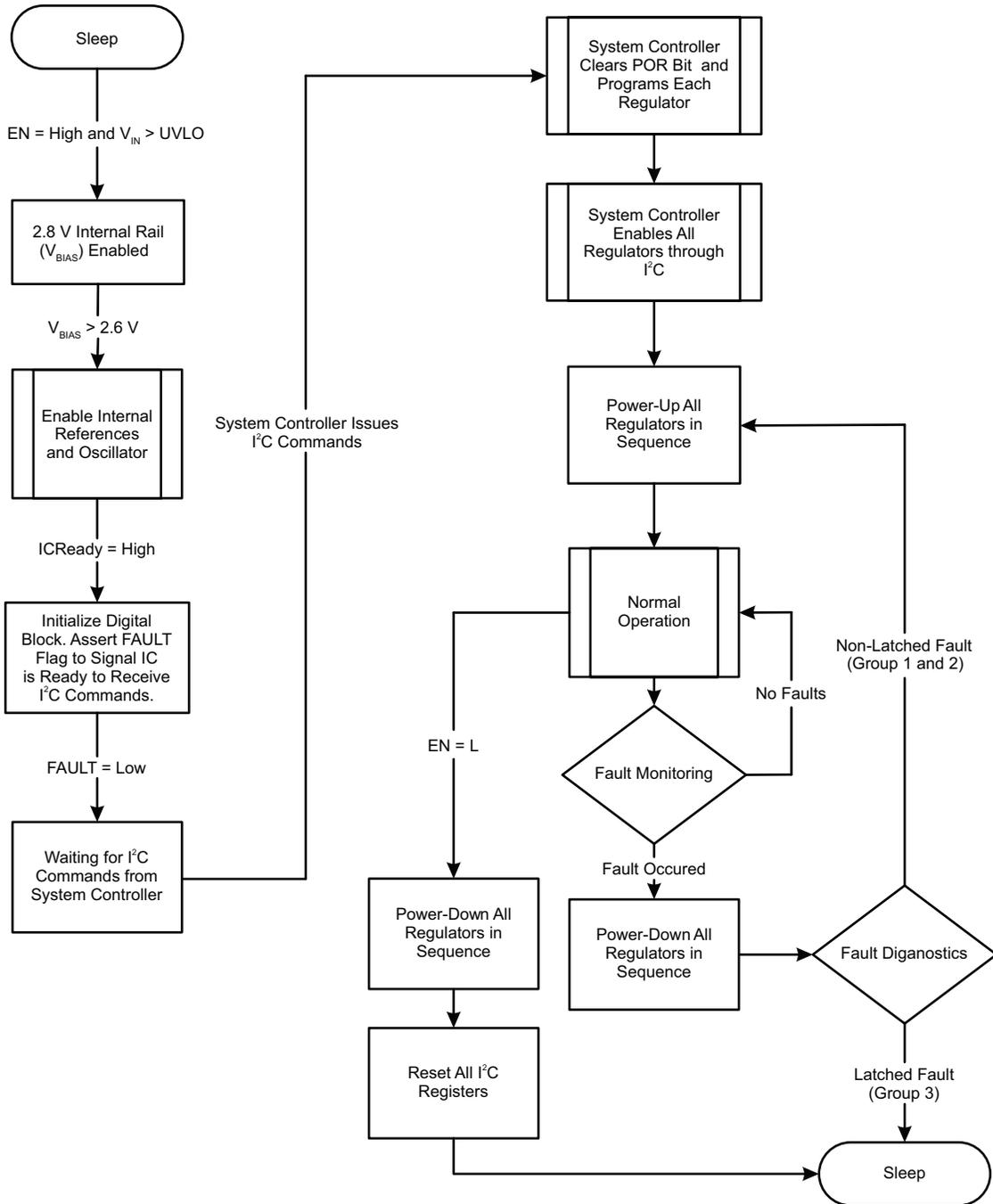
Figure 17: Fault Checking During Startup and Normal Operation
