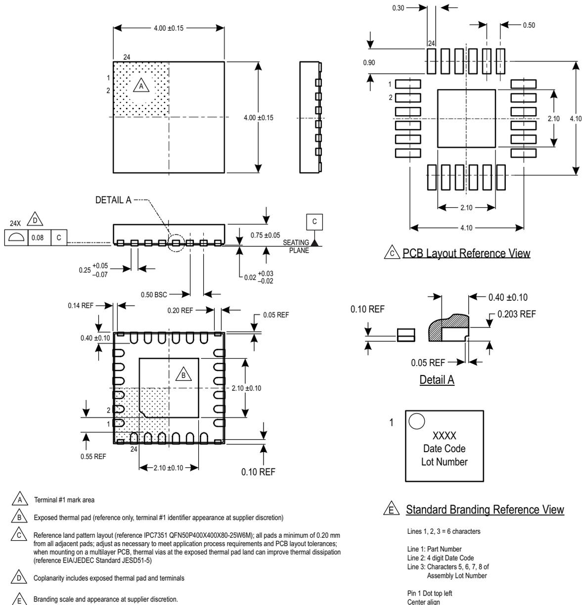
Figure 21: Package ES, 24-Pin 4 mm × 4 mm QFN with Exposed Thermal Pad and Wettable Flank
