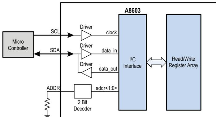
**Figure 1: I<sup>2</sup>C Serial Interface and Programmable Memory Array**
