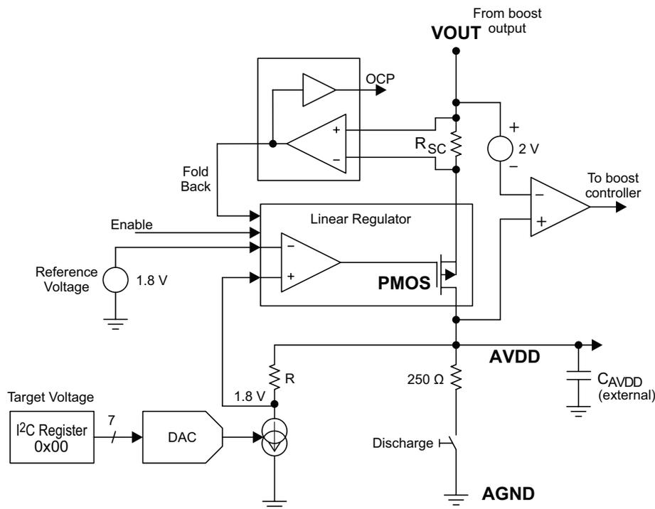
Figure 3: Representative Block Diagram of the AVDD Regulator
