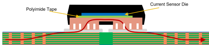
Figure 16: No Vias Under Copper Pads (not to scale)
