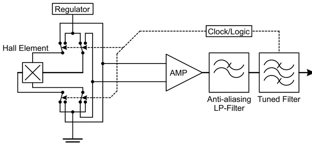
Figure 5: Concept of Chopper Stabilization Technique
