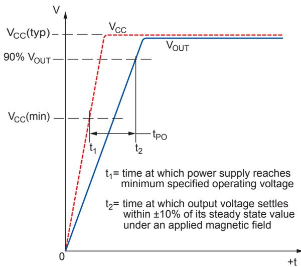
Figure 1. Definition of Power On Time,  $t_{PO}$
