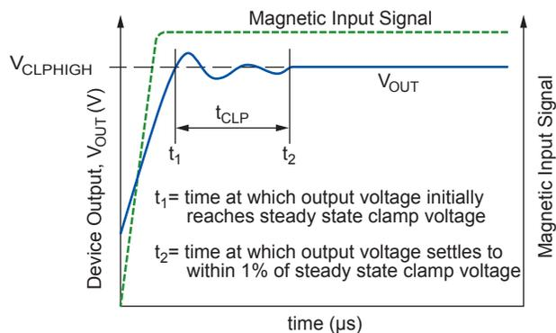
Figure 2. Definition of Delay to Clamp,  $t_{CLP}$
