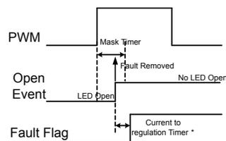
\* Current to regulation timer is 256 switching cycles.
