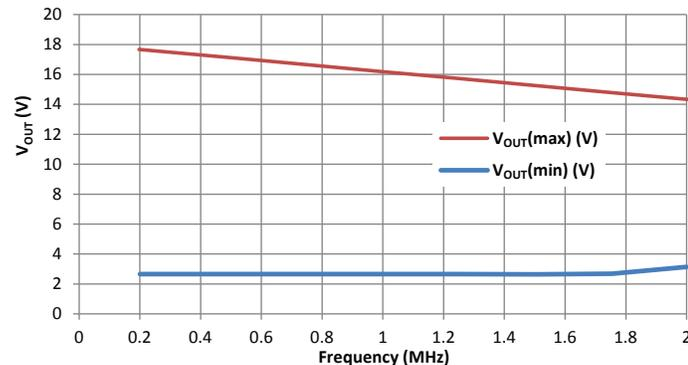
**Figure 11: Minimum and Maximum Output Voltage vs. Switching Frequency**
