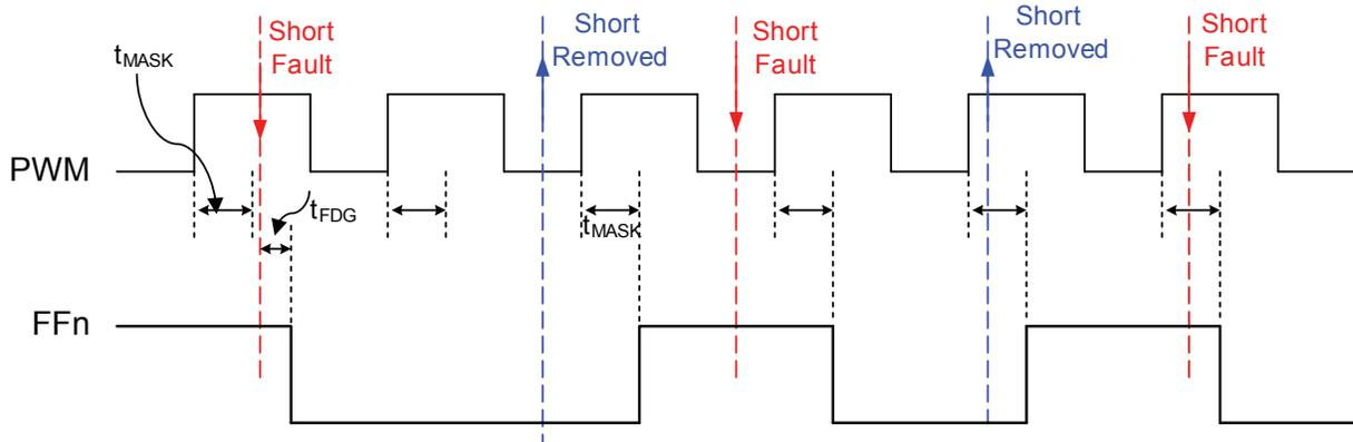
Figure 13a: LED Short Fault Timing Diagram Overview
