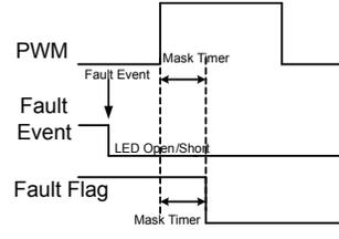
**Case 5: LED Open/Short Removed at PWM = L**
