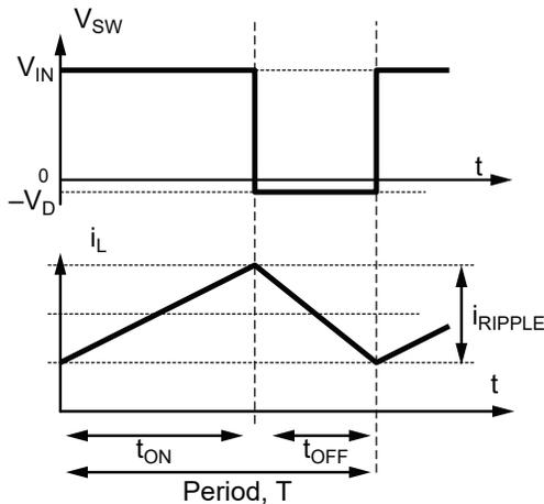
Note:  $V_D = R_{DSON(LS)} \times i_L$
