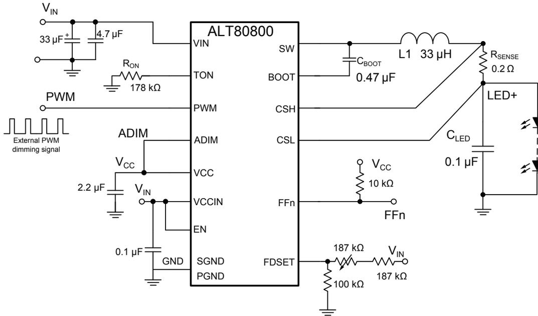
Figure 18: Application Circuit Example for ALT80800
