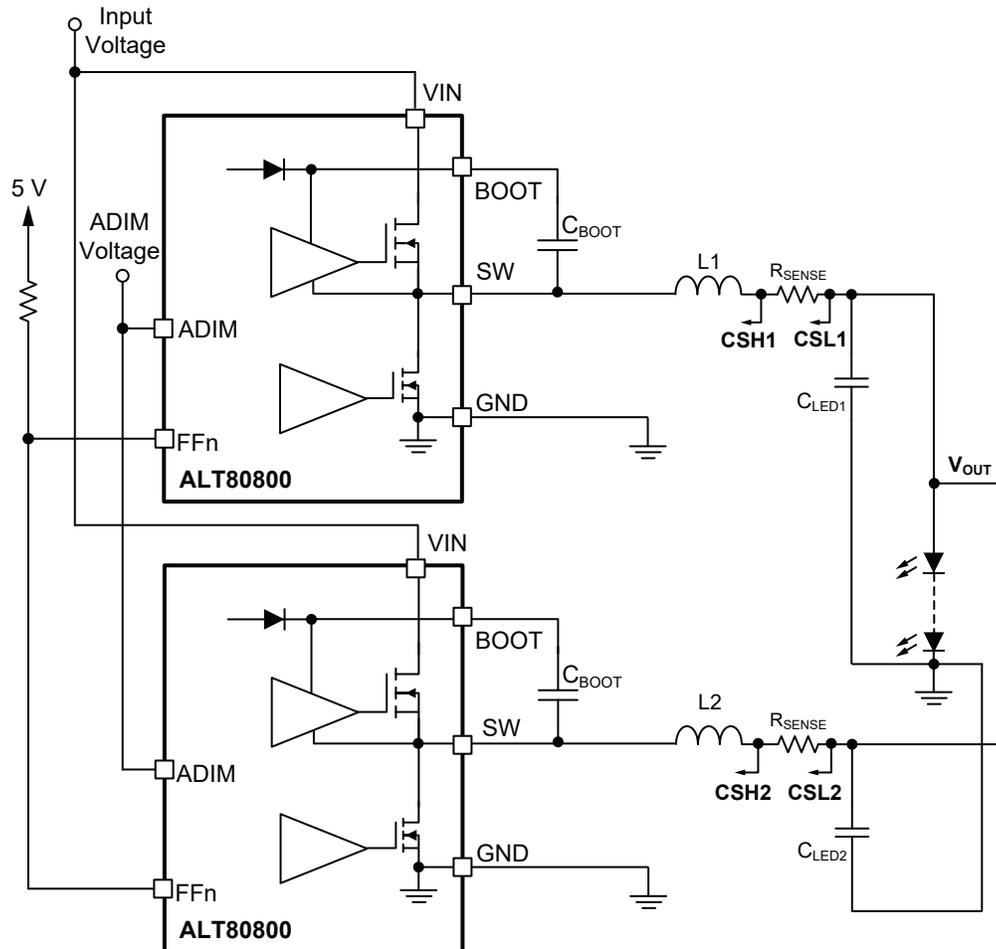
Figure 19: Using 2 (or more) ALT80800 in parallel to drive the same LED string.
