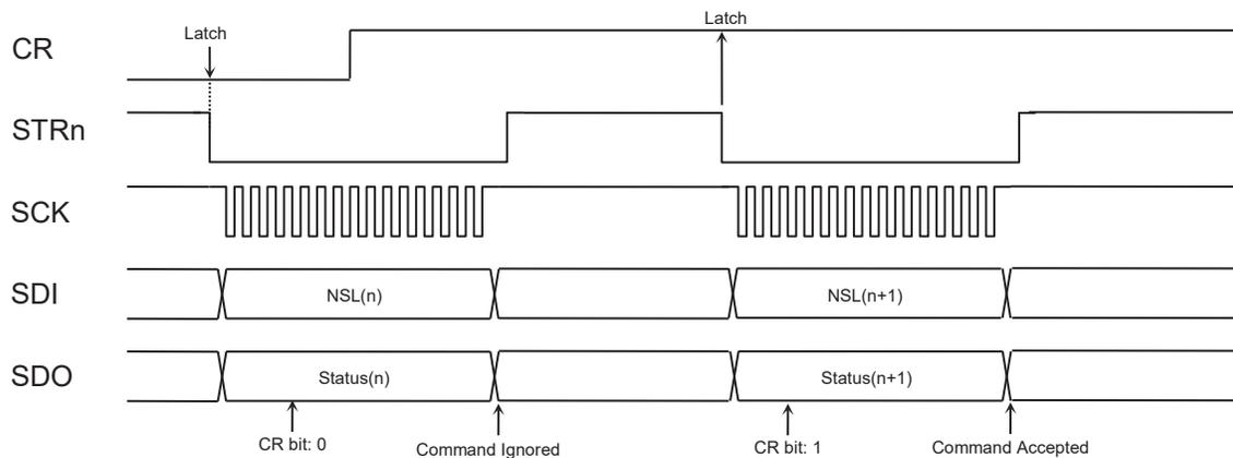
**Figure 24: Motion Profile Update with CR Status Checking**
