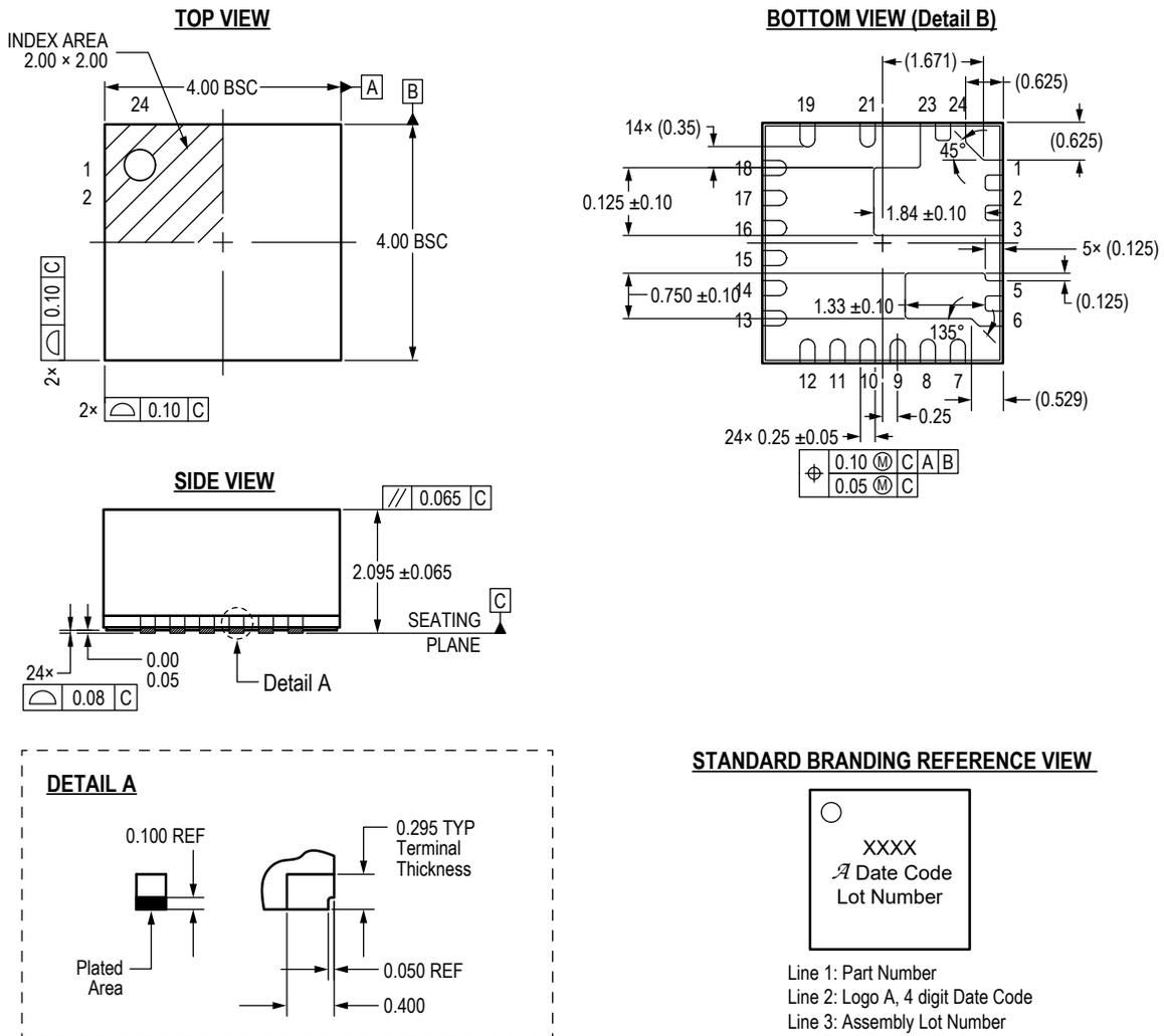
Figure 15: 24-Lead 4 mm × 4mm QFN (Suffix NB)
