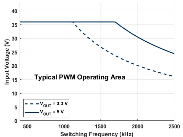
Figure 8: Input Voltage Limit To Prevent Pulse Skipping
