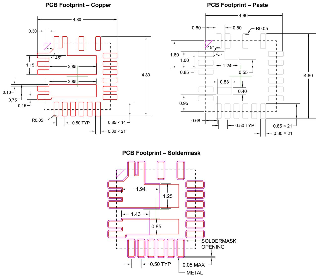
**Figure 16: Recommended PCB Footprint**
