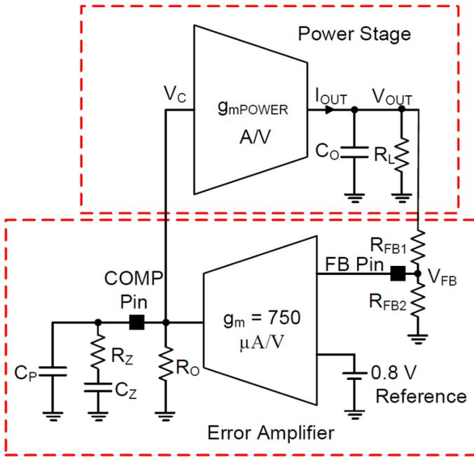
**Figure 11: Power Stage and Error Amplifier**
