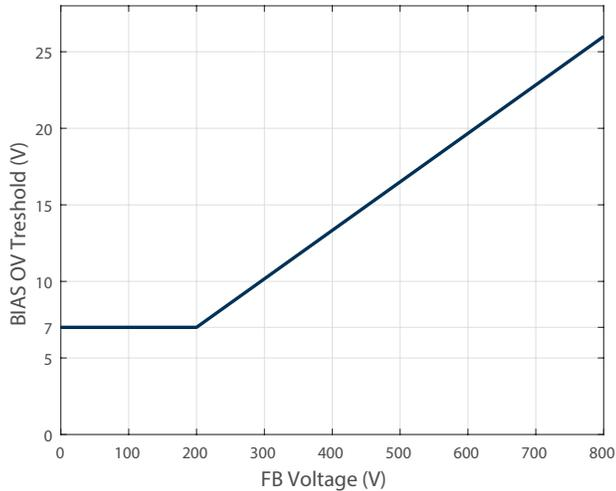
**Figure 6: BIAS Overvoltage Threshold vs. FB Pin Voltage**
