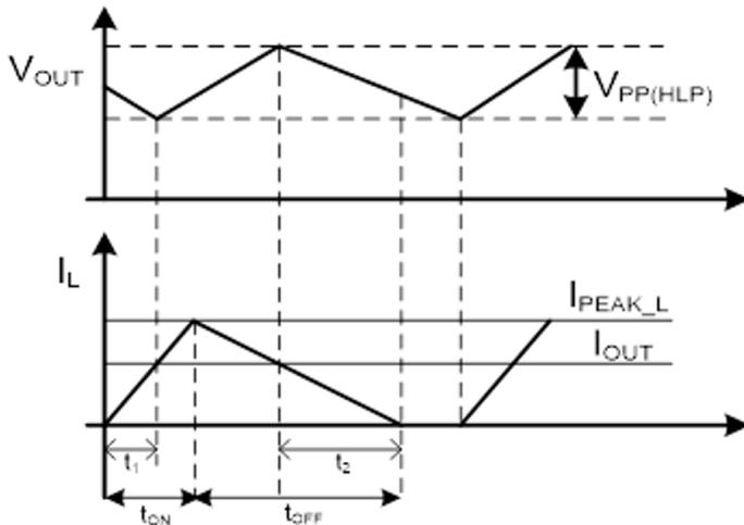
**Figure 9: Output Voltage Ripple in LP Mode**
