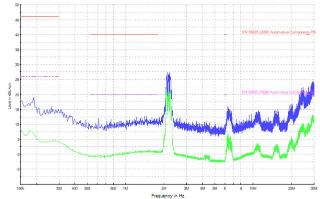
**Radiated Emissions (150 kHz to 30 MHz) (Monopole)**
