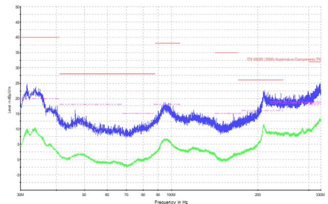
**Radiated Emissions (30 MHz to 330 MHz)
