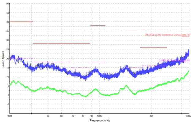
**Radiated Emissions (30 MHz to 330 MHz)
